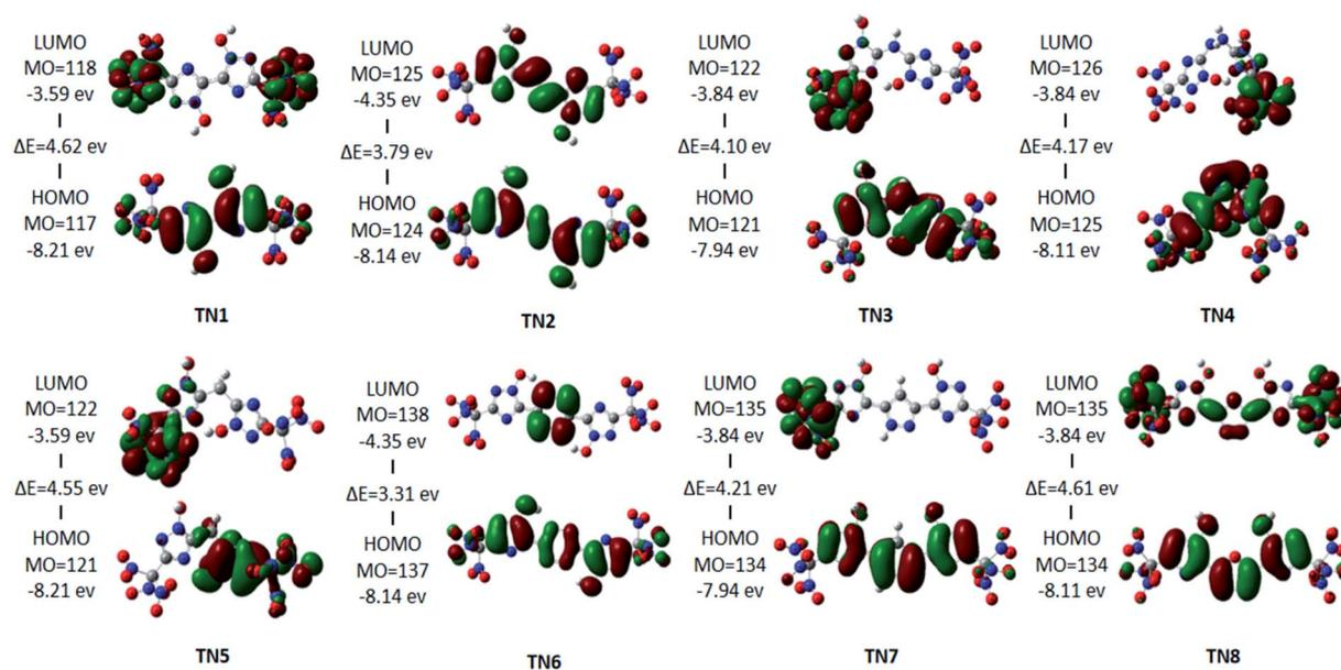
Fig. 3 HOMO-LUMO orbitals and HOMO-LUMO energy gap of the  $-\text{C}(\text{NO}_2)_3$  (TN) series.
