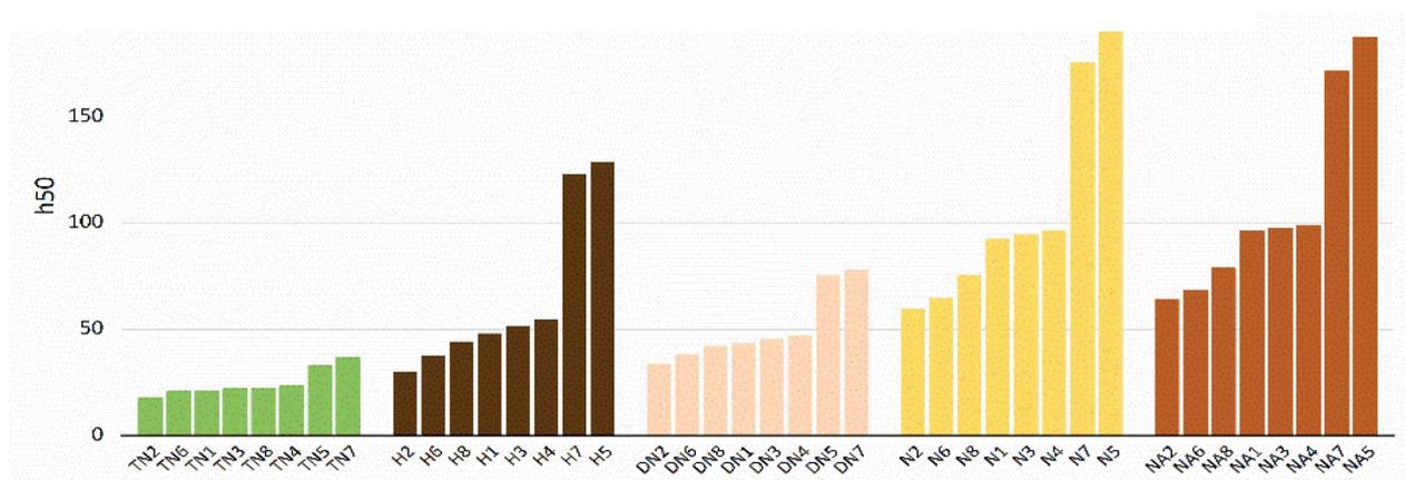
Fig. 13 Impact sensitivities ( $h_{50}$ ) sorted by substituted groups  $-\text{C}(\text{NO}_2)_3$  (TN),  $-\text{OH}$  (H),  $-\text{C}(\text{NO}_2)_2$  (DN),  $-\text{NO}_2$  (N),  $-\text{NHNO}_2$  (NA).
