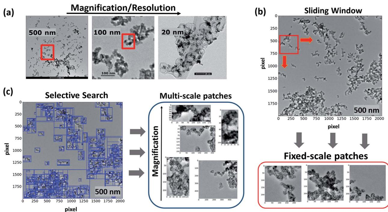
**Fig. 1** (a) An example of real-world images of catalyst ink agglomerates at different magnification levels or resolutions. (b) Representation of the sliding window technique to sample fixed-scale patches from high-resolution TEM images of catalyst inks. (c) Representation of the selective search algorithm<sup>57</sup> to sample patches from high-resolution TEM images of inks based on hierarchical grouping of similar regions such as color, size, texture, and shape compatibility.
