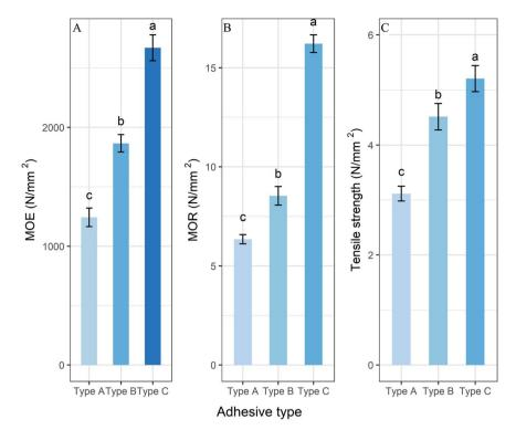
Fig. 2 Modulus of elasticity (MOE) (A), modulus of rupture (MOR) (B) and tensile strength (C) of jute stick-based particleboards (JSPs) with different NRL-based bio-adhesive formulae (see Table 1).
