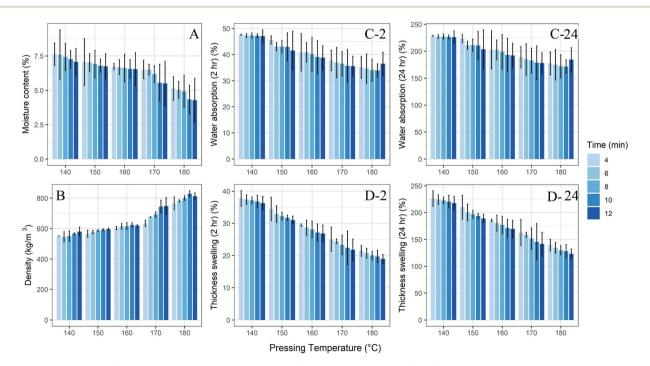
Fig. 4 Moisture content (A), density (B), water absorption after two (C-2) and twenty-four (C-24) hour, and thickness swelling after two (D-2) and twenty-four (D-24) hour of type C particleboards.
