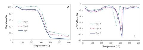
Fig. 3 Thermogravimetric analysis (TGA) (A) and derivative thermogravimetry (DTG) (B) performance of the jute stick particleboards (JSPs) produced from three types (Table 1) of NRL-based bio-adhesive formula. Thermoanalysis was carried out under nitrogen atmosphere using a heating rate of 10 °C min<sup>-1</sup> according to ASTM E1582.<sup>45</sup>
