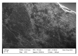
Fig. 6 A SEM micrograph of the type C JSP pressing at 180  $^{\circ}$ C temperature for 8 min.
