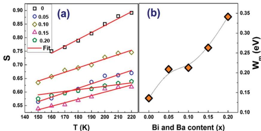
Fig. 13 (a) Variation of the exponent of Jonscher's power law  $S$  vs.  $T$  and (b) the  $W_m$  activation energies of the  $\text{La}_{1-2x}\text{Bi}_x\text{Ba}_x\text{FeO}_3$  ( $x = 0.0, 0.05, 0.1, 0.15$  and  $0.2$ ) compounds.
