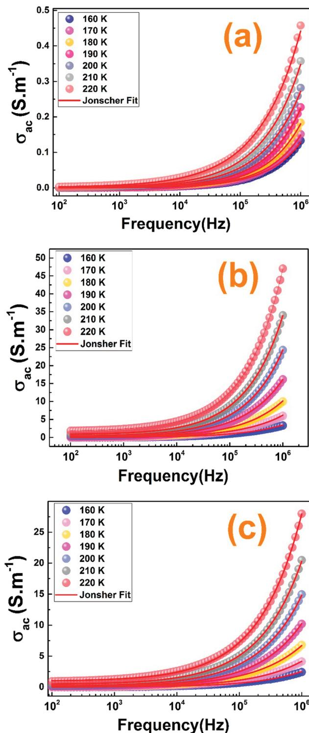
Fig. 12 (a–c) The ac-conductivity adjustment results with the Jonscher's power law of the  $\text{La}_{1-2x}\text{Ba}_x\text{Bi}_x\text{FeO}_3$  ( $x = 0.00, 0.10$  and  $0.20$ ) compounds, respectively.
