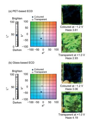
Fig. 5 Variation in CIELAB colour coordinates ( $L^*$ ,  $a^*$ ,  $b^*$ ) and photographs of the (a) PET-based and (b) glass-based ECDs in the colored and transparent states.
