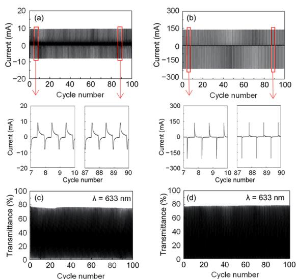
Fig. 6 Cycle stability up to 100 cycles of (a and c) PET-based and (b and d) glass-based ECDs illustrated as (a and b) MPS measurements of electrochemical stability at constant voltages of  $-1.2$  and  $+1.0$  V, and (c and d) transmittance at a wavelength of  $633$  nm.
