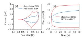
Fig. 3 (a) CV and (b) CC profiles of the glass-based (red) and PET-based (blue) ECDs acquired at a potential scan rate of 5 mV s $^{-1}$ .
