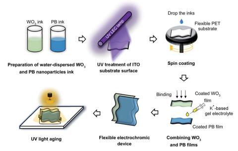
Fig. 1 Schematic of ECD preparation.
