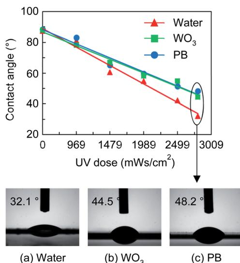
Fig. 2 Contact angles for water and the PB and  $\text{WO}_3$  inks dropped on the ITO/PET substrate after UV treatment at various UV irradiation intensities. The photos show the contact angle of (a) water, (b)  $\text{WO}_3$ , and (c) PB on the surface of ITO-coated PET substrate treated with a UV dose of  $2805 \text{ mW s cm}^{-2}$ .
