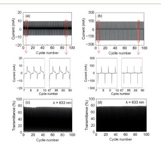
Fig. 6 Cycle stability up to 100 cycles of (a and c) PET-based and (b and d) glass-based ECDs illustrated as (a and b) MPS measurements of electrochemical stability at constant voltages of -1.2 and +1.0 V, and (c and d) transmittance at a wavelength of 633 nm.
