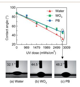
Fig. 2 Contact angles for water and the PB and  $WO_3$  inks dropped on the ITO/PET substrate after UV treatment at various UV irradiation intensities. The photos show the contact angle of (a) water, (b)  $WO_3$ , and (c) PB on the surface of ITO-coated PET substrate treated with a UV dose of 2805 mW s cm<sup>-2</sup>.
