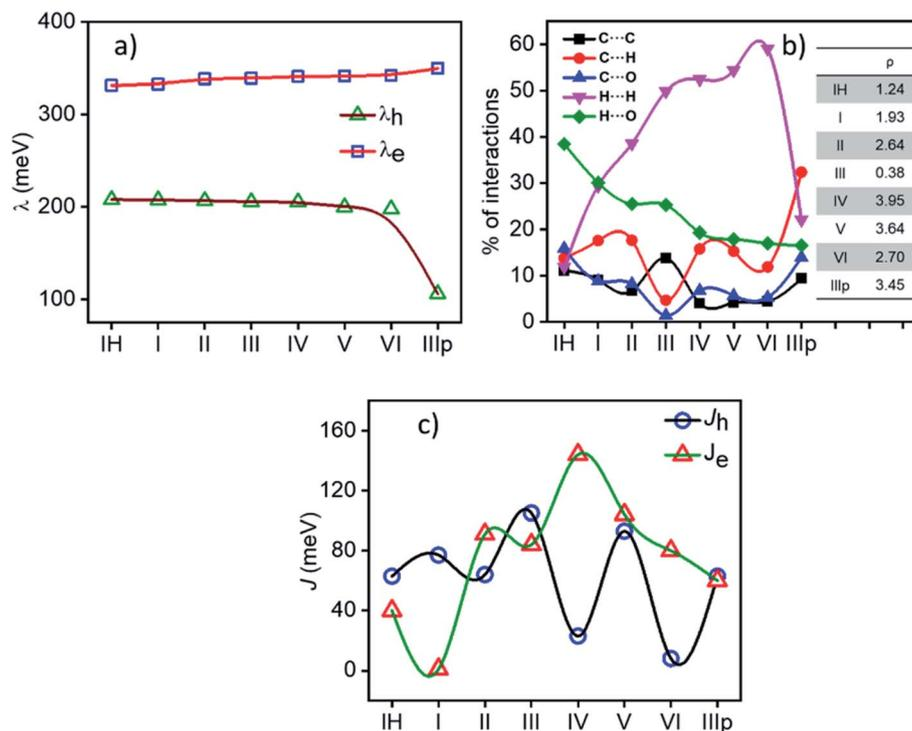
Fig. 3 (a) Variation in internal reorganization energy of the NDIs under consideration. (b) Percentage of non-covalent interactions obtained from the Hirshfeld surface analysis (values of  $\rho[(\% \text{C}\cdots\text{H})/(\% \text{C}\cdots\text{C})]$  are shown in the inset). (c) Hole and electron charge transfer integrals along the M–D1 pair of NDIs.
