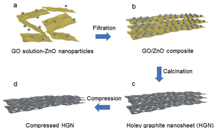
Fig. 10 The synthesis approach to produce holey graphene sheets from GO using ZnO nanoparticles. Reprinted with permission.<sup>80</sup> Copyright 2018, Royal Society of Chemistry.
