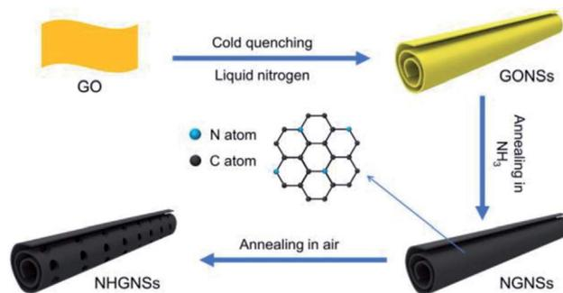
Fig. 7 Schematic picture showing the steps to prepare HG nanoscrolls, as demonstrated by Su *et al.* Reprinted with permission.<sup>65</sup> Copyright 2021, Elsevier.
