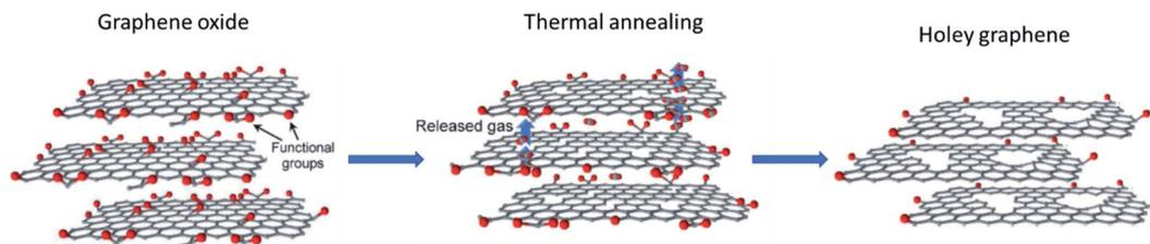
Fig. 5 Schematic representation of the formation of holey graphene from graphene oxide using rapid thermal annealing. Reprinted and adapted with permission.<sup>66</sup> Copyright 2015, John Wiley and Sons.
