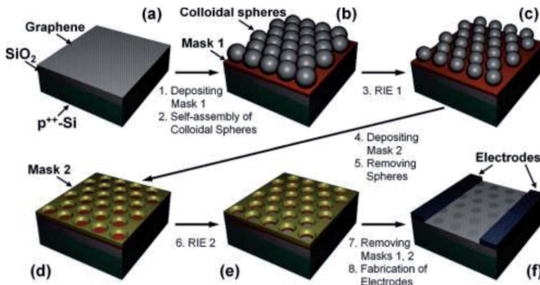
Fig. 17 Schematic of the nanomesh fabrication process using colloidal microspheres and RIE. Reprinted with permission.<sup>107</sup> Copyright 2010, American Chemical Society.
