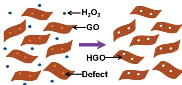
Fig. 14 A schematic diagram to describe the synthesis process of HGO. Reprinted with permission.<sup>87</sup> Copyright 2015, American Chemical Society.
