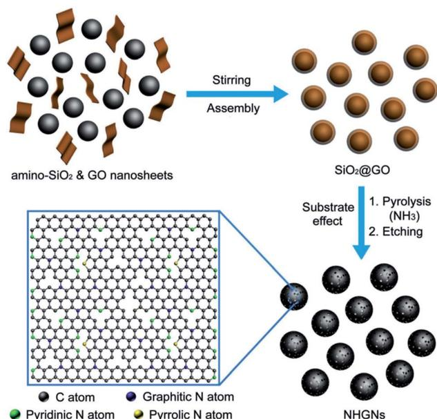
Fig. 16 Schematic figure showing the steps for the synthesis of NHGNs. Reprinted with permission.<sup>104</sup> Copyright 2016, John Wiley and Sons.
