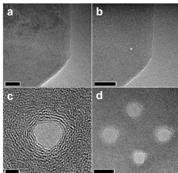
Fig. 4 TEM images of a graphene sheet (a) before and (b) after an energetic electron beam makes a nanopore. (c) Higher magnification image of the nanopore. (d) Multiple nanopores are made close to each other. Scale bars are 50, 50, 2, and 10 nm, respectively. Reprinted and adapted with permission.<sup>48</sup> Copyright 2008, AIP Publishing.
