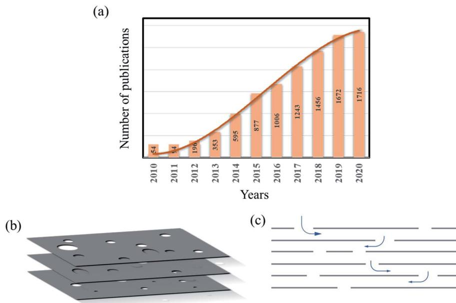
**Fig. 1** (a) The chart shows the number of publications focused on holey/porous graphene in the last ten years (data obtained from Scopus). (b) The schematic image shows the presence of nanoscale pores in a stack of graphene sheets. (c) The cross-sectional schematic view shows the interlayer channels formed in a stack of graphene sheets due to randomly distributed pores. Ions or molecules with sizes lower than the pore sizes could pass through the material (shown by the arrows).
