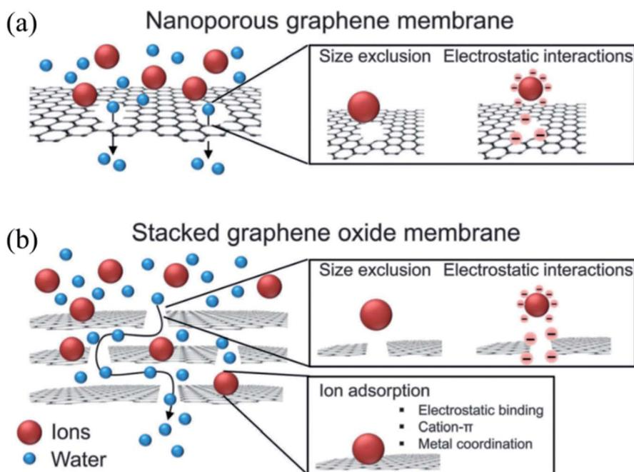
Fig. 20 Water purification via ion filtering using nanoporous graphene (a) and stacked graphene oxide (b). Reprinted with permission.<sup>33</sup> Copyright 2015, Royal Society of Chemistry.
