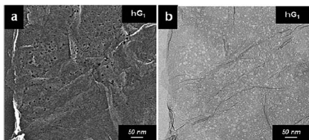
Fig. 9 Electron microscopy images of a holey graphene sample prepared using Ag nanoparticles as the catalyst. Reprinted with permission.<sup>77</sup> Copyright 2013, Royal Society of Chemistry.
