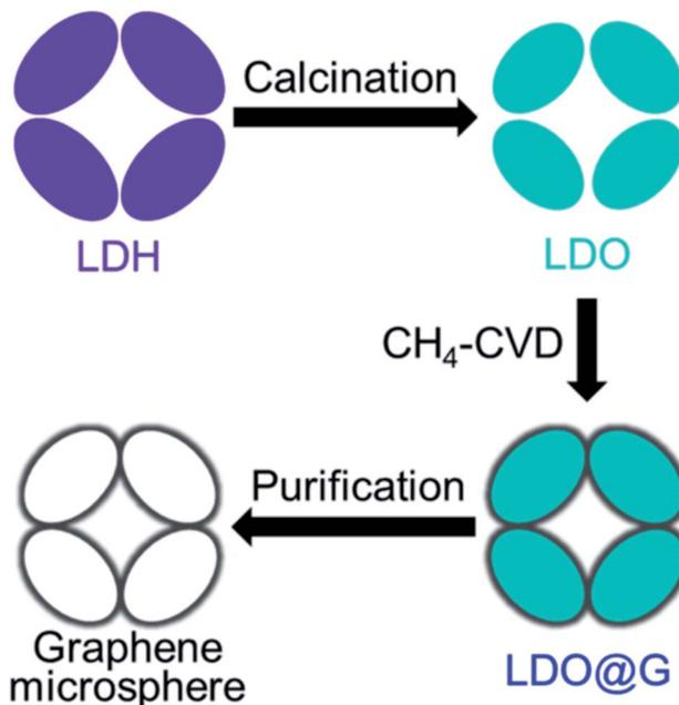
Fig. 18 Schematic picture indicating the steps to grow graphene microspheres. Reprinted with permission.<sup>109</sup> Copyright 2015, Elsevier.
