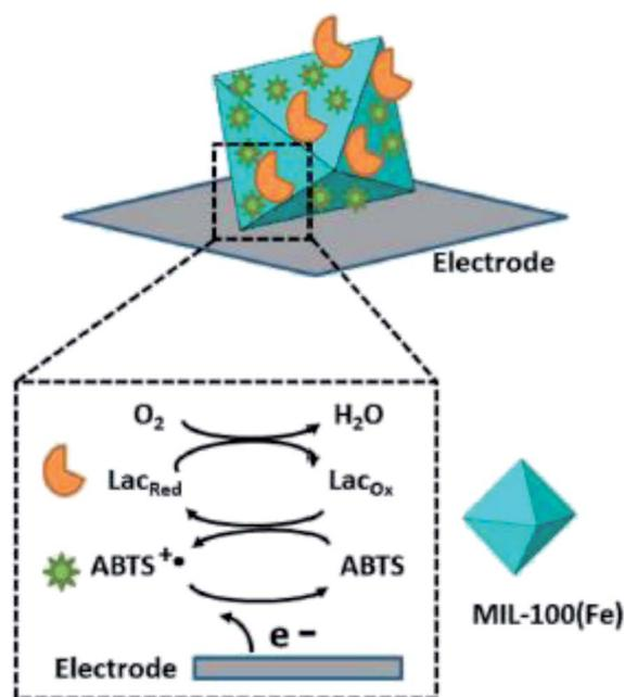
Fig. 6 MIL-100(Fe) immobilized laccase-ABTS by impregnated adsorption.<sup>44</sup>
