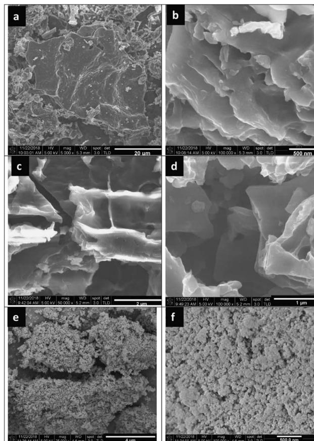
Fig. 10 FESEM images of (a and b) samples obtained after the carbonization of tea waste at 650 °C, (c and d) the synthesized rGO, and (e and f) the nanocomposite of GO/TiO<sub>2</sub>. These figures have been reproduced from ref. 117 with permission from IOPscience, copyright: 2020.
