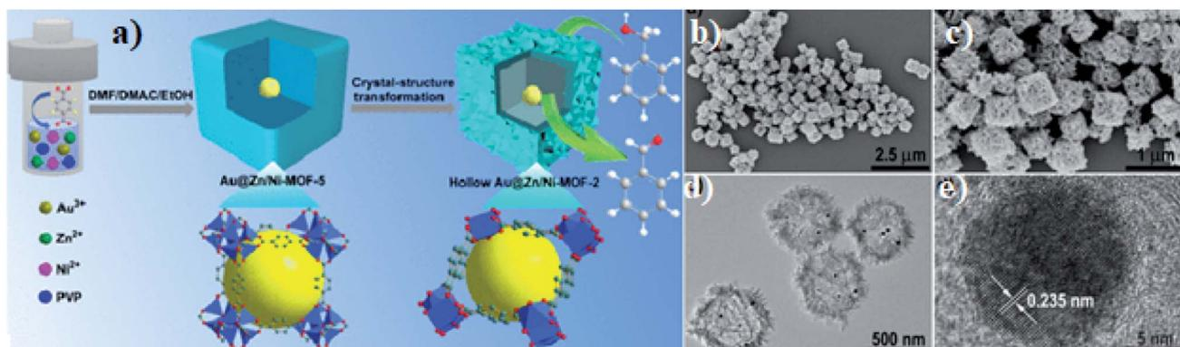
**Fig. 7** (a) Scheme of preparation of a hollow Au@Zn/Ni-MOF-2 core-shell nanoreactor, (b and c) SEM and (d and e) TEM of hollow Au@Zn/Ni-MOF-2 core-shell nanocubes. Reproduced from ref. 81 with permission from American Chemical Society, Copyright 2021.
