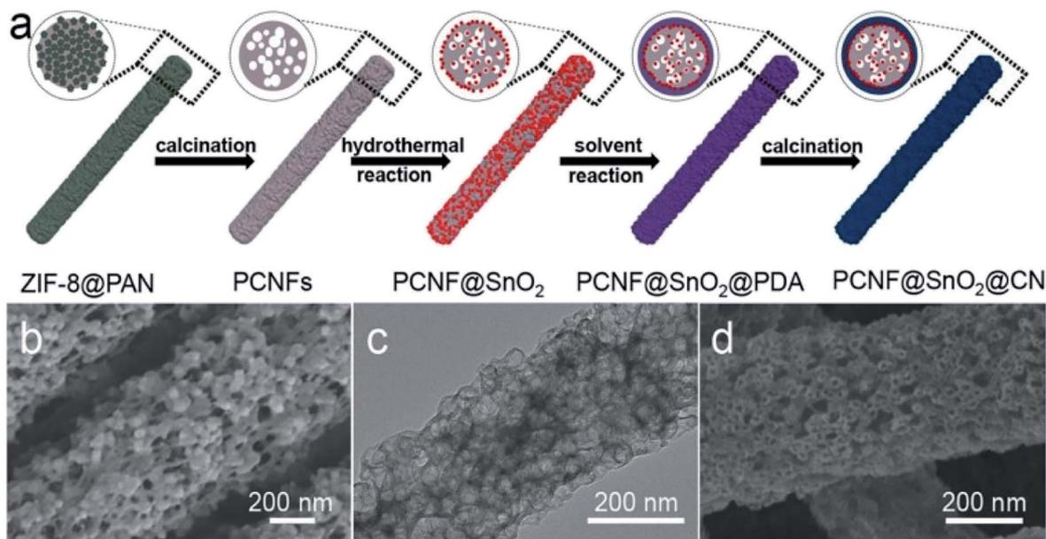
Fig. 8 (a) Schematic illustration of the preparation of PCNF@SnO<sub>2</sub>@CN nanofibers, (b) SEM and (c) TEM of PCNF nanofibers, (d) SEM of PCNF@SnO<sub>2</sub>@CN nanofibers. Reproduced from ref. 83 with permission from Elsevier, Copyright 2021.
