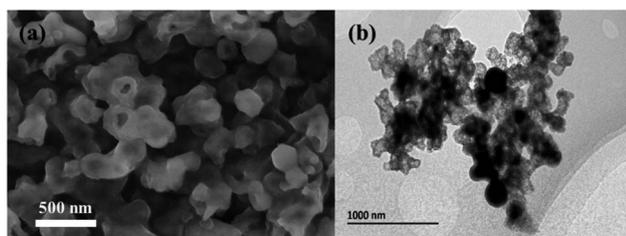
Fig. 9 (a) SEM and (b) TEM of ZnSe/MoSe<sub>2</sub>@C showing a well-defined polyhedral structure. Reproduced from ref. 83 with permission from Royal Society of Chemistry, Copyright 2019.
