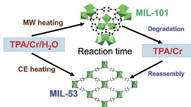
Fig. 4 Various morphologies of MOFs obtained by tuning reaction conditions. Reproduced from ref. 63 with permission from Royal Society of Chemistry, Copyright 2018.
