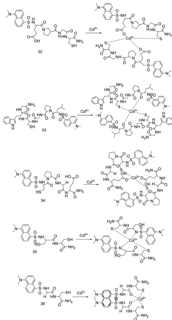
Fig. 12 The probes structure reported by P. Wang's team and proposed binding mode with Cd<sup>2+</sup>.
