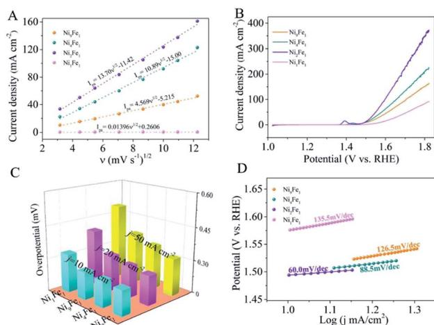
Fig. 3 Electrochemical tests for the OER performance of various NiFe-LDHs samples in  $1\text{ M KOH}$  solution. (A) Linear correlation between the  $I_{pa}$  and the  $\nu^{1/2}$ . (B) Polarization curves and (C) the overpotentials required for different current densities and (D) corresponding Tafel plots.
