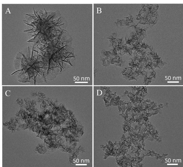
Fig. 1 TEM images of various NiFe-LDHs samples prepared at room temperature by the co-precipitation method: (A)  $\text{Ni}_9\text{Fe}_1$ -LDHs, (B)  $\text{Ni}_4\text{Fe}_1$ -LDHs, (C)  $\text{Ni}_2\text{Fe}_1$ -LDHs and (D)  $\text{Ni}_1\text{Fe}_1$ -LDHs.
