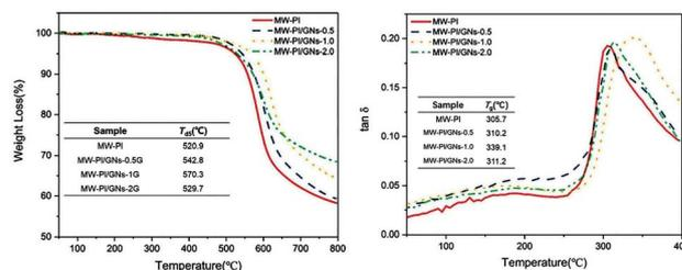
Fig. 6 The TGA curves and DMA curves of MW-PI/GNs fibers with different GNs content.
