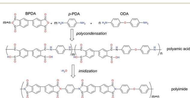
Scheme 1 Synthetic process of BPDA/*p*-PDA/ODA co-PI.
