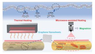
Fig. 1 Structure and preparation process of PI/GNs fibers.
