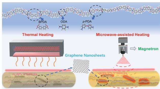
Fig. 1 Structure and preparation process of PI/GNs fibers.
