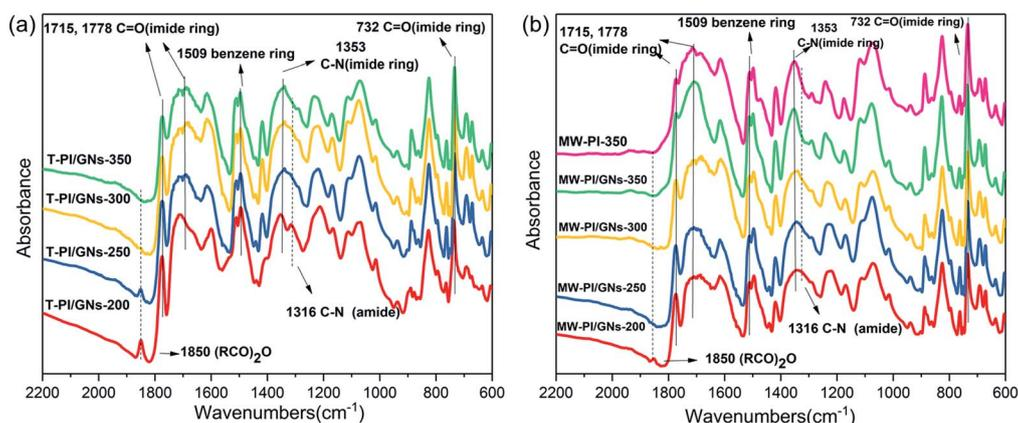
Fig. 2 FT-IR spectra of the PI/GNs fibers ((a) T-PI/GNs; (b) MW-PI/GNs).
