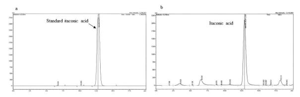
Fig. 1 Chromatogram of organic acid with the main component of commercial (a) and bio-synthetic itaconic acids (b). Sample was injected through Aminex HPX-87H (300 mm  $\times$  7.8 mm) columns. Conditions: mobile phase, 0.005 N sulfuric acid; flow rate, 1 mL min<sup>-1</sup>; column temperature, 60 °C; and detection, refractive index.
