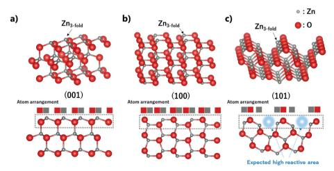
Fig. 7 Crystallographic structure, side view, and atom arrangement of (002), (100), and (101) planes of Zn.
