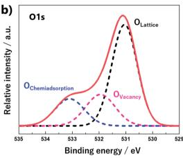
**Fig. 8** High-resolution XPS spectra of (a) Zn 2p and (b) O 1s for ZnO nano-bullet.
