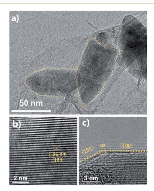
Fig. 5 (a) TEM image and (b and c) HR-TEM image of ZnO nanobullets synthesized by solution plasma.
