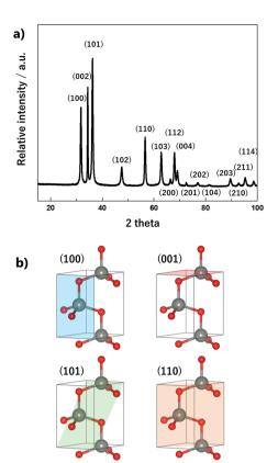
Fig. 6 (a) XRD patterns of ZnO nano-bullets and (b) representative crystallographic planes of ZnO.
