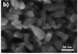
Fig. 4 (a and b) Morphology of ZnO nano-bullet synthesized by solution plasma
