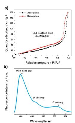
Fig. 9 Isotherm curve with the (a) BET surface area and (b) fluorescence spectrum of the ZnO nano-bullet.
