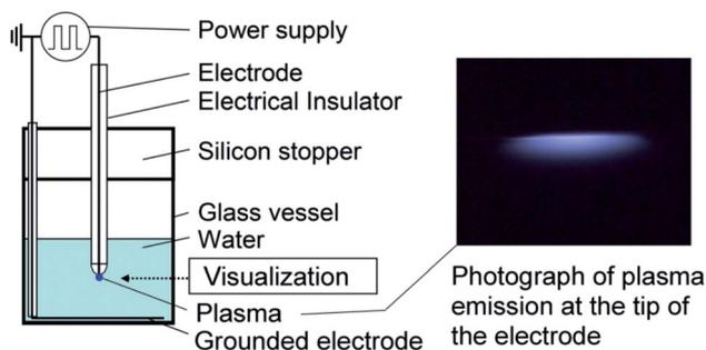
Fig. 18 Schematic of the experimental setup to form bulk nanobubbles *via* plasma generation in a specific volume of water. The plasma forms between the electrode tip placed in the water and the grounded electrode after turning on the high-voltage power supply.<sup>137</sup>
