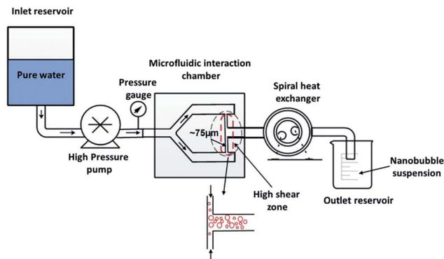
Fig. 11 The experimental setup with the integration of a Y-type microfluidic cell used by Nirmalkar *et al.* for the generation of bulk nanobubbles.<sup>12</sup>
