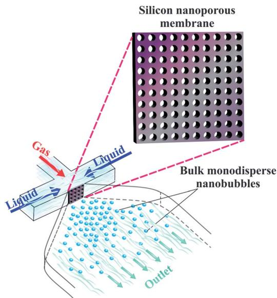
Fig. 24 Production of bulk monodisperse nanobubbles via an embedded silicone nanoporous membrane in a PDMS microfluidic chip.
