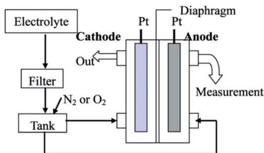
Fig. 17 Production of bulk nanobubbles through the electrolysis technique. An electrolyte solution passes from a filter with 100 nm holes before being merged with gas ( $\text{O}_2$  or  $\text{N}_2$ ) in the tank. Then, the mixed solution with gas in the tank transports to the chamber where the electrodes are placed. The electric current passing from the electrode anode to the cathode electrode electrolyzes the water inside the chamber.<sup>134</sup>
