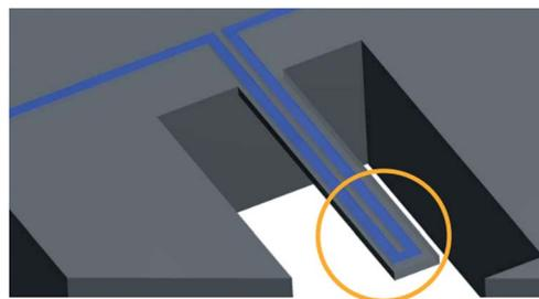
Fig. 6 An embedded microchannel in a silicon microcantilever. The circled section highlights the tip of the microcantilever where the sensitivity is maximum.<sup>98</sup>
