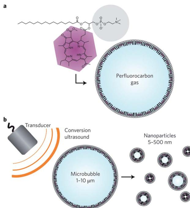
Fig. 16 Bulk nanobubbles generation *via* fragmentation of microbubbles. (a) A microbubble consists of bacteriochlorophyll-lipid and perfluorocarbon gas. (b) Production of bulk nanobubbles through applying low-frequency ultrasound to the bacteriochlorophyll-lipid shell microbubbles.<sup>132</sup>
