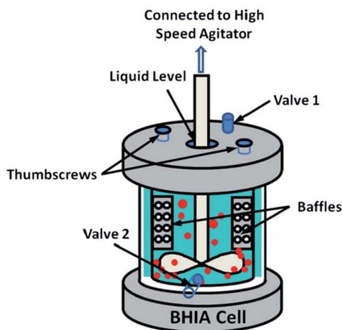
Fig. 9 Baffled high-intensity agitation (BHIA) cell used by Wu *et al.* to generate bulk nanobubbles. After introducing the solution into a baffled cell, the rotating impeller connected to a high-speed agitator creates hydrodynamic cavitation leading to the generation of bulk nanobubbles. Valves 1 and 2 are used to take samples for the characterization of the generated bulk nanobubbles. The thumbscrews are placed to tightly seal the cap cell to the cell body.<sup>118</sup>
