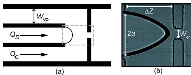
Fig. 22 Microbubble production by flow focusing. (a) A schematic drawing, and (b) microscopic image of flow focusing geometries. In (a),  $Q_D$ ,  $Q_C$ , and  $W_{up}$  represent the gas flow rate, liquid flow rate, and distance between the device wall and the gas channel, respectively. In (b), the orifice width, the gas flow channel width, and the junction-to-orifice distance is shown by  $W_{or}$ ,  $2a$ , and  $\Delta Z$ , respectively.<sup>154</sup>
