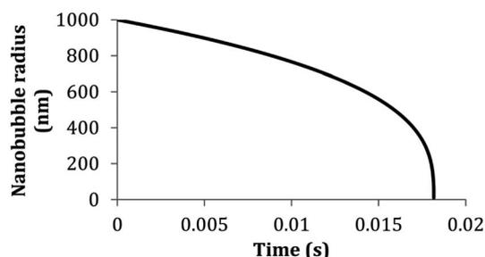
Fig. 1 Lifetime of a bubble smaller than 1000 nm predicted by the theory of Epstein and Plesset. The graph depicts the calculated radius of a nitrogen-filled bubble in a nitrogen saturated solution *versus* time ( $T = 300$  K,  $\gamma = 0.072$  J m<sup>-2</sup>,  $D = 2.0 \times 10^{-9}$  m<sup>2</sup> s<sup>-1</sup>,  $C_{\text{sat}} = 0.6379$  mol m<sup>-3</sup>,  $\rho_{1 \text{ atm}} = 40.6921$  mol m<sup>-3</sup>).<sup>8,9</sup>
