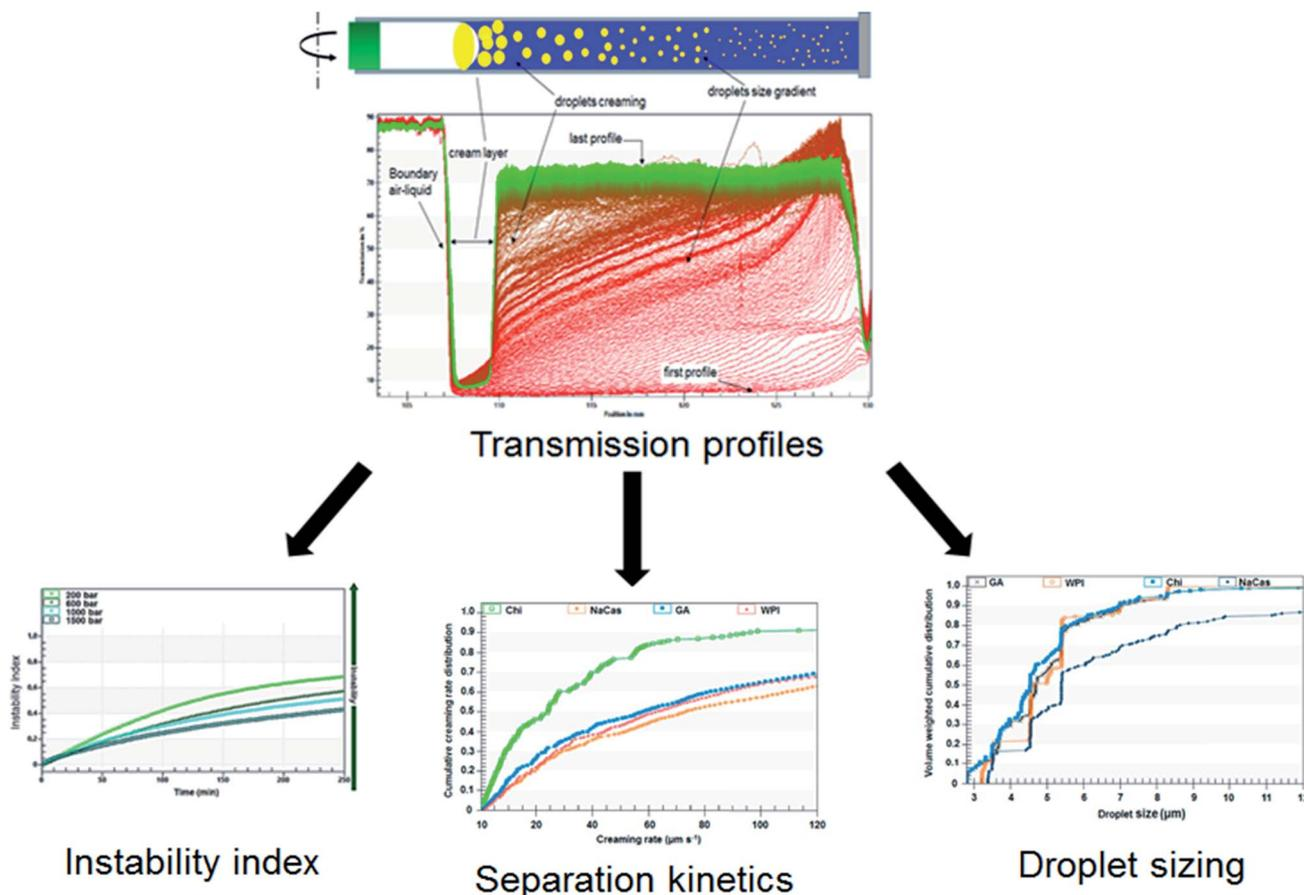
Fig. 1 Schema of accelerated stability evaluation of emulsions using LUMiSizer® analytical centrifugation test.<sup>54,55</sup>
