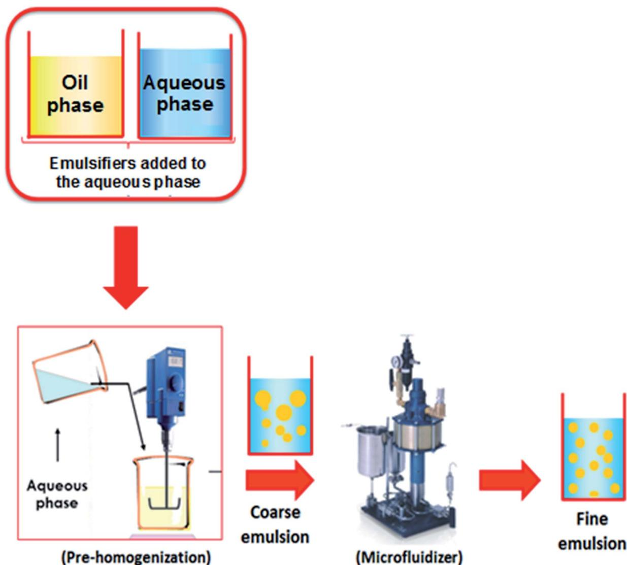
Fig. 3 Nanoemulsions elaboration using two-step emulsification method.<sup>46</sup>
