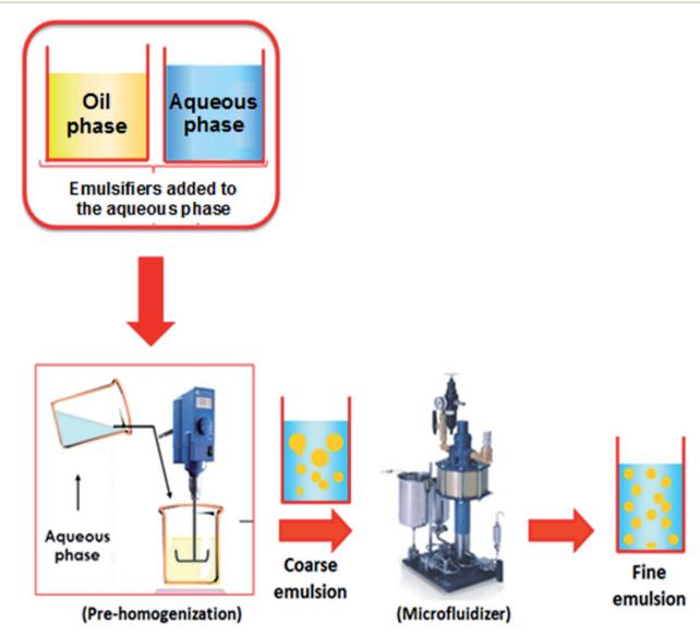
Fig. 3 Nanoemulsions elaboration using two-step emulsification method. 46
