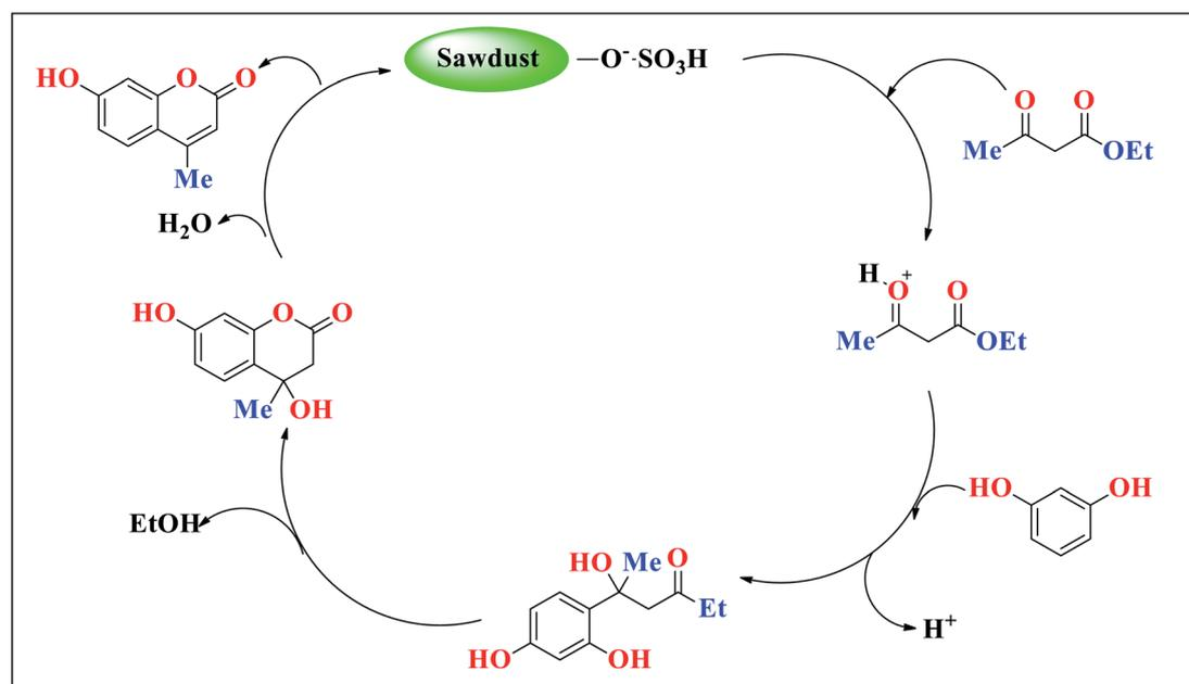
**Fig. 14** The plausible mechanism of formation of 7-hydroxy-4-methylcoumarin in presence of sulfonated sawdust (SD-SO<sub>3</sub>H) as solid acid catalyst.
