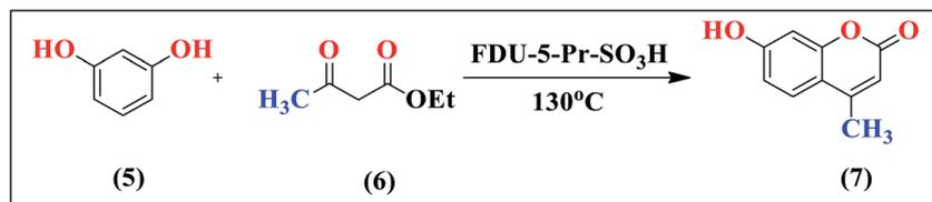
Scheme 14 Synthesis of coumarin derivatives via Pechmann condensation of phenols with  $\beta$ -keto-ester catalyzed by FDU-5-Pr-SO<sub>3</sub>H.
