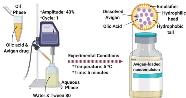
Fig. 3 The process of preparing Avigan-loaded nano-emulsions.
