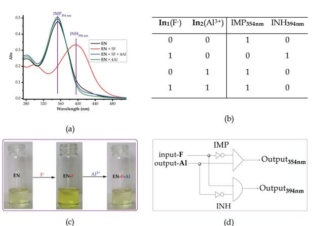
Fig. 11 (a) Absorption spectra of EN ( $1 \times 10^{-5}$  M) in DMSO- $H_2O$  with  $F^-$  and the molecular logic functions "IMP" (354 nm) and "INH" (394 nm), (b) truth table, (c) reversible and reproducible colorimetric activities and (d) schematic representation of a combinatorial IMP/INH logic circuit.
