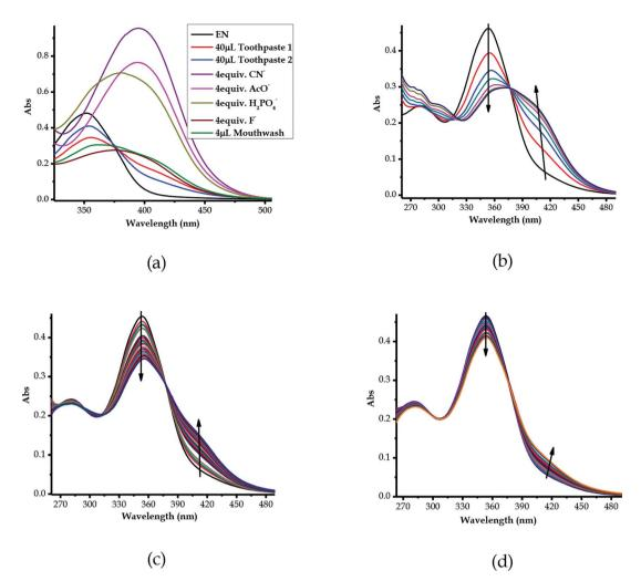
Fig. 12 UV-vis spectra of EN (1  $\times$  10<sup>-5</sup> M) in DMSO-H<sub>2</sub>O: (a) combined absorption spectra of the different anions, (b) mouthwash (4  $\mu$ L), (c) toothpaste 1 (20  $\mu$ L) and (d) toothpaste 2 (20  $\mu$ L) upon the addition of drops of the toothpaste solutions (20g ml<sup>-1</sup>) in H<sub>2</sub>O.
