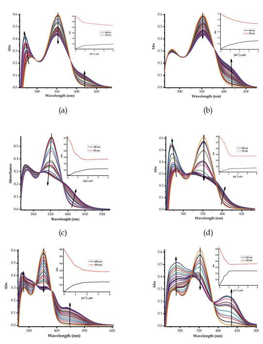
Fig. 3 The absorption titration spectra of EN (1  $\times$  10<sup>-5</sup> M) in DMSO-H<sub>2</sub>O upon the addition of 5 equiv. of (a) Pb<sup>2+</sup>, (b) Sn<sup>2+</sup>, (c) Ag<sup>+</sup>, (d) Hg<sup>2+</sup>, (e) Co<sup>2+</sup> and (f) Cu<sup>2+</sup> (0.03 M) at room temperature, with their titration profiles shown in the insets.
