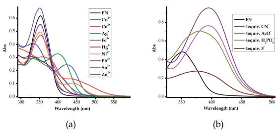
Fig. 14 Combined absorption spectra of EN (1  $\times$  10<sup>-5</sup> M) in DMSO-H<sub>2</sub>O, after titrated with, (a) 2 equiv. of the cations and (b) 4 equiv. of the anions
