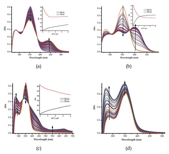
Fig. 4 The absorption titration spectra of EN  $(1 \times 10^{-5} \text{ M})$  in DMSO- $H_2O$  upon the addition of 5 equiv. of (a) Ni<sup>2+</sup>, (b) Zn<sup>2+</sup>, (c) Fe<sup>2+</sup> and (d) Fe<sup>3+</sup> (0.03 M) at room temperature, with their titration profiles shown in the insets.
