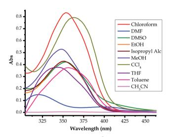
Fig. 8 Absorption spectra of EN (1 imes 10 $^{-5}$  M) in different solvents for solvatochromism, at room temperature.
