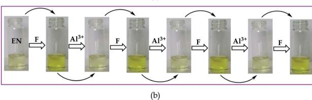
Fig. 10 Reversible cycles and reproducible colorimetric switch of EN (1  $\times$  10<sup>-5</sup> M, DMSO-H<sub>2</sub>O) reversed and reproduced by the addition of F and Al $^{3+}$ , respectively, (a) repeating cycles and (b) colorimetric switch of up to 4 cycles.
