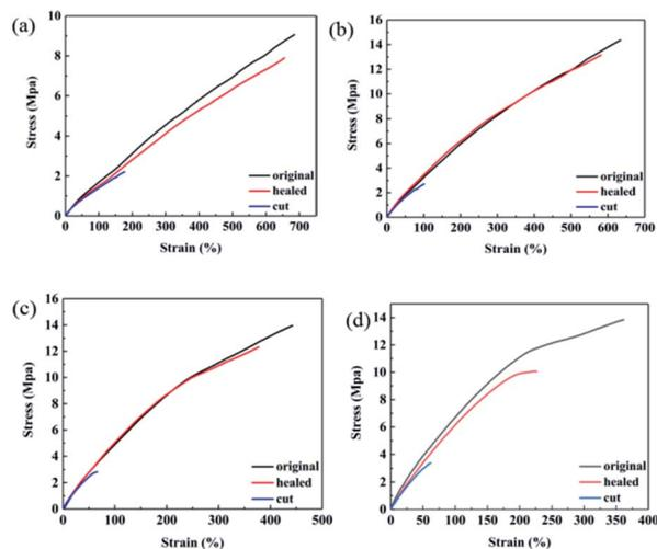
Fig. 5 Stress–strain curves of samples with different  $-NCO/-OH$  ratios.
