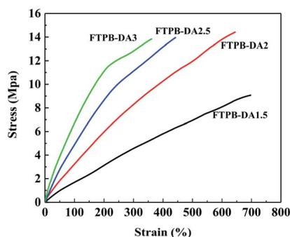
Fig. 4 Comparison of the mechanical properties of FTPB-DA with different  $-NCO/-OH$  ratio.
