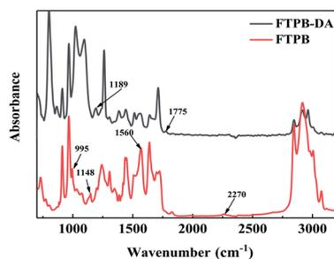
Fig. 1 FTIR spectra of FTPB and FTPB-DA.
