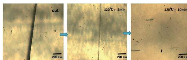
Fig. 3 POM images of a crack in FTPB-DA2 during the healing process.
