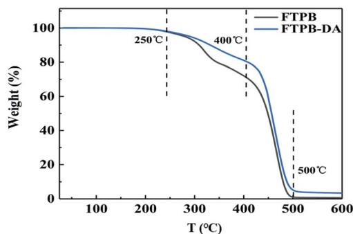
Fig. 8 The TGA curves of FTPB and FTPB-DA.
