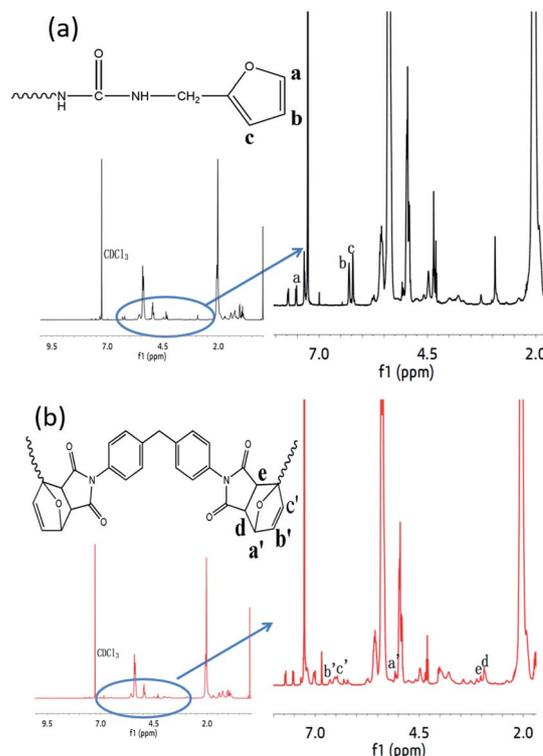
Fig. 2 (a) <sup>1</sup>H-NMR spectra of FTPB (b) <sup>1</sup>H-NMR spectra FTPB-DA.
