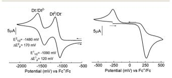
Fig. 2 Cyclic voltammograms of  $\bf 6$  at a scan rate of 100 mV s $^{-1}$ . Experimental details are included with the physical methods of the ESI.†
