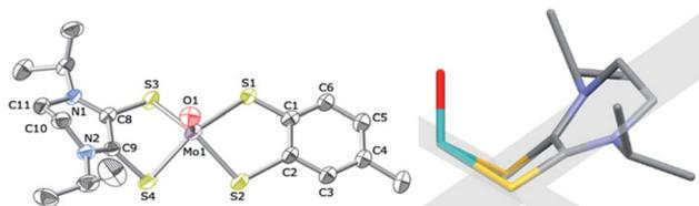
Fig. 1 Left: thermal ellipsoid plot (30%) of  $[\text{MoO}(\text{tdt})({}^i\text{Pr}_2\text{Dt}^0)]$ . Space group,  $Pbca$ ;  $R_1$ , 0.054;  $wR_2$ , 0.100. Right: schematic demonstrating the drastic fold angle along the SS vector (defined by intersecting planes shown in grey) of the  ${}^i\text{Pr}_2\text{Dt}^0$  ligand of **6**. Crystallographic details are listed in Table S1.†
