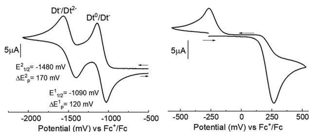
Fig. 2 Cyclic voltammograms of **6** at a scan rate of 100 mV s<sup>-1</sup>. Experimental details are included with the physical methods of the ESI.†
