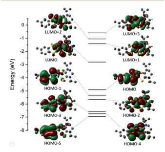
Fig. 3 Energy diagram and corresponding molecular orbitals for 6.
