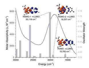
Fig. 4 Calculated transitions (bars) imposed on experimental UV-Vis data of 6. PCM-TDDFT calculations were done using MeCN as the solvent to match experimental conditions. Transitions for the low energy band are paired with their corresponding electron density differential map (EDDM). Electron donating orbitals are blue and electron accepting orbitals are orange.
