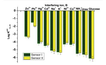
Fig. 6 Selectivity coefficient pattern for copper-paper selective electrodes based on ionophores I and II.
