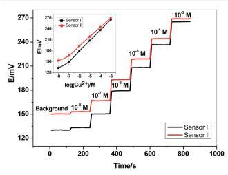
Fig. 3 The potentiometric response and time-trace for Cu<sup>2+</sup>-paper based sensors.
