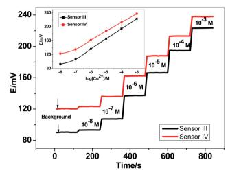
Fig. 4 The potentiometric response and time-trace for GC/Cu<sup>2+</sup>-based sensors.
