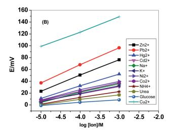
Fig. 5 Selectivity pattern for the paper-based electrochemical device based on (A) sensor I and (B) sensor II.
