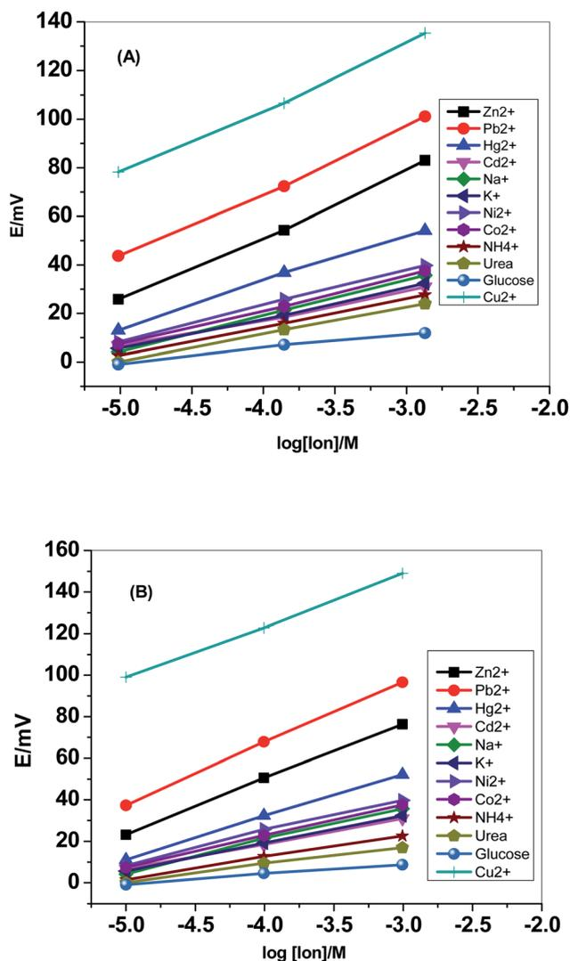
Fig. 5 Selectivity pattern for the paper-based electrochemical device based on (A) sensor I and (B) sensor II.
