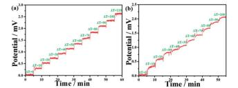
Fig. 5 V-T curves of the s-Cu<sub>2-x</sub>Se sample under heating (a) and cooling (b) processes, respectively.
