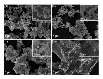
Fig. 2 SEM images of (a) CuSe, (b)  $Cu_3Se_2$ , (c)  $Cu_{2-x}Se$ , and (d) s- $Cu_{2-x}Se.$
