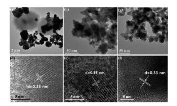
Fig. 3 TEM and HRTEM images of CuSe (a and d), Cu<sub>3</sub>Se<sub>2</sub> (b and e) and  $Cu_{2-x}Se$  (c and f), respectively.
