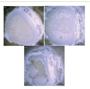
Fig. 8 Oxidized surface in different PECO time: (a)  $5 \, \text{s}$ , (b)  $10 \, \text{s}$  and (c)  $30 \, \text{s}$ .
