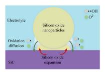
Fig. 10 Schematic illustration of SiO<sub>2</sub> nanoparticle formation.
