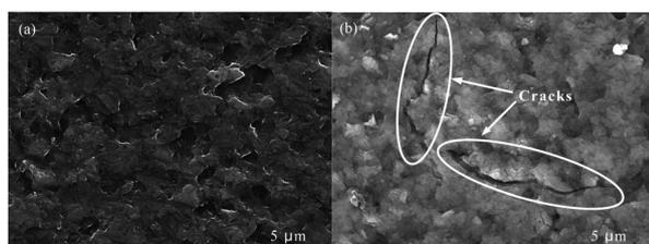
Fig. 3 Surface morphology of SiC surface before and after oxidation: (a) as-received surface, (b) PECO processed surface.
