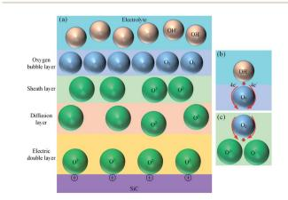
Fig. 1 SiC-solution interface and formation process of  $O^{2-}$ : (a) SiC-solution interface, (b) oxygen film accumulates on SiC surface, (c)  $O^{2-}$  formation.
