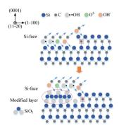
Fig. 9 Schematic diagram of interface chemical reaction on Si-face.
