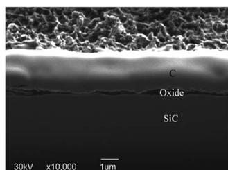
Fig. 7 Cross section image of oxidized sample.
