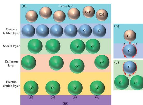
Fig. 1 SiC-solution interface and formation process of O<sup>2-</sup>: (a) SiC-solution interface, (b) oxygen film accumulates on SiC surface, (c) O<sup>2-</sup> formation.
