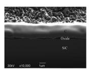
Fig. 7 Cross section image of oxidized sample.
