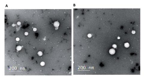
Fig. 2 Transmission electron micrograph of the prepared LPH NPs. Both  $LPH_{Azi-Pir}$  (A) and  $LPH_{Nic-Pir}$  (B) appeared as a core-shell structure with particle size 120–130 which agreed with the size obtained by dynamic light scattering.
