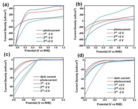
Fig. 4 LSV curves of CdS/BTO NWs samples under light irradiation with twice -3 V followed by once +3 V polarizations in (a) positive voltage section (-0.1 V to +1.2 V) and (c) negative voltage section (0.2 V to -0.8 V). And the LSV curves with twice +3 V followed by once -3 V polarizations in (b) positive voltage section and (d) negative voltage section.
