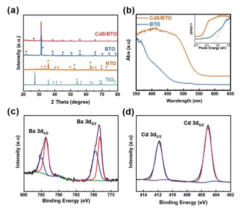
Fig. 2 (a) XRD patterns of the  $TiO_2$ , NTO, BTO and CdS/BTO NWs samples. (b) UV-vis absorption spectra and the inset in (b) presents the corresponding plots of  $(\alpha h v)^2$  vs. photon energy. XPS spectra of the CdS/BTO NWs samples: (c) Ba 3d and (d) Cd 3d peaks.
