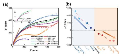
Fig. 5 (a) EIS Nyquist plots of the CdS/BTO NWs samples after different polarizations and the inset shows the results for -3 V ( $2^{\text{nd}}$ ). Open circles were test data points and solid lines were corresponding fitting. (b) Impedance change value compared to unpolarized sample of the CdS/BTO NWs samples.
