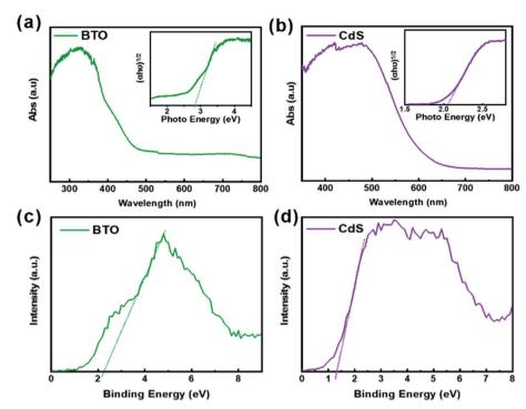
Fig. 8 UV-vis absorption spectra of (a) BTO and (b) CdS. The insets in (a and b) present the corresponding plots of  $(\alpha h \nu)^2 vs$ . photon energy. Valence-band XPS spectra of (c) the BTO and (d) CdS samples.
