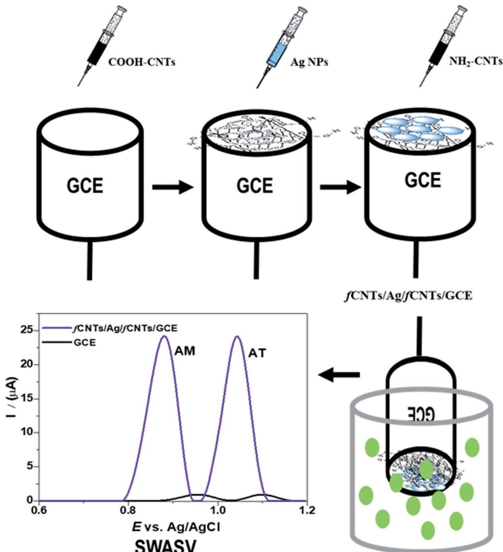
Scheme 1 The fabrication and application of COOH-CNTs/Ag/NH<sub>2</sub>-CNTs nanocomposite sensor.
