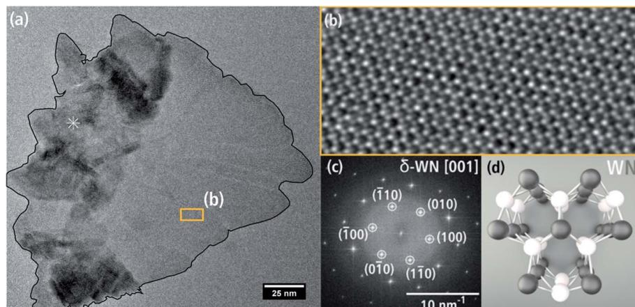
Fig. 7 (a) Bright-field TEM image of a sheet aggregate (left side) bordering a single  $\text{WN}_x$  sheet and (b) HRTEM image from the region of the single sheet marked in (a). (c) Shows the FT of (b) and is indexed with the hexagonal  $\delta\text{-WN}_x$  structure. A model of this crystal structure in [001] zone-axis orientation is shown in (d).
