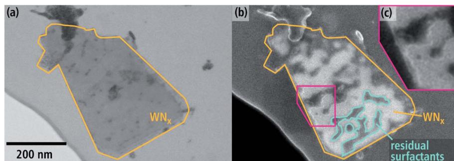
**Fig. 4**  $WN_x$  nanosheet with several inhomogeneities visible in (a) BF-STEM and (b) SE-SEM images taken from the same region at 30 keV in a scanning electron microscope. (c) Shows a magnified region of (b).
