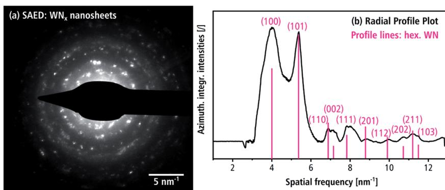
Fig. 8 (a) SAED pattern of agglomerated  $\text{WN}_x$  nanosheets with beam stop blocking the zero-order beam and (b) the corresponding azimuthally integrated intensity plot with Bragg reflections for  $\delta\text{-WN}$  with hexagonal structure. The pink lines indicate the calculated positions and kinematic intensities of the Bragg reflections for the  $\delta\text{-WN}_x$  structure.
