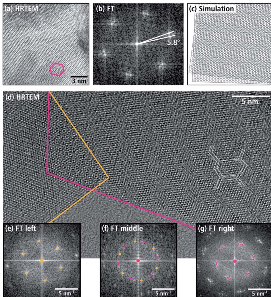
**Fig. 9** (a) TEM image of stacked  $\text{WN}_x$  nanosheets, which show a honeycomb moiré pattern. (b) FT image of the moiré pattern area in (a). The pattern in (a) was simulated in (c) with a simple graphics program. (d) HRTEM image of an edge region of several stacked sheets with a complex moiré pattern (red) and a single sheet below (yellow). (e and g) FT images of the red and yellow marked area in (d), and (f) FT image of the overlap region.
