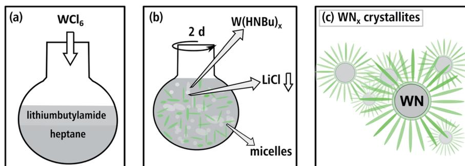
Fig. 1 Illustration of the synthesis route for batch a in (a) and (b), where  $W(HNBu)_x$  and a micellar template are formed. (c) The soft sacrificial template produces small aggregated  $WN_x$  crystallites.
