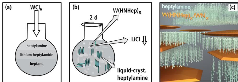
Fig. 2 Illustration of the synthesis route for batch b in (a) and (b), where  $W(\text{HNHep})_x$  and a liquid-crystalline phase is formed. (c) Shows a model of the lateral crystal growth mechanism of  $W(\text{HNHep})_x$  and  $W\text{N}_x$ .
