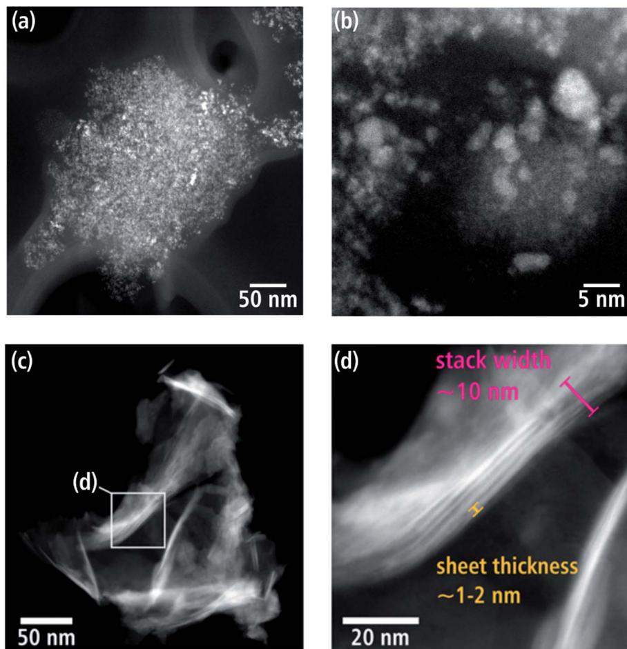
**Fig. 3** (a) HAADF-STEM overview image of a  $WN_x$  aggregate (batch (a) and (b)) image taken at larger magnification. (c) HAADF-STEM overview of  $WN_x$  nanosheets (batch (b)). The region indicated with a white square is shown enlarged in (d). A stack of nanosheets with a thickness of 1–2 nm is marked in (d).
