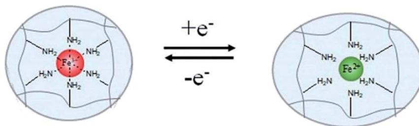
Fig. 12 Mechanism of shape memory effect and rapid reversible actuation of hydrogels with electrochemically controlled local metal ion coordination and crosslinking.<sup>123</sup> Copyright 2020. Reproduced with permission from Royal Society of Chemistry.
