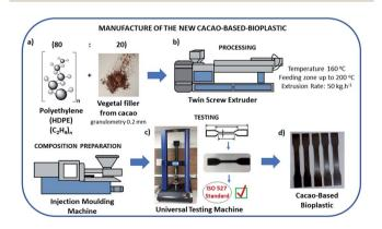
Fig. 1 Manufacturing process of new cacao-based bioplastic. (a) The bioplastic was manufactured using high density polyethylene (HDPE) and cacao shells as vegetal filler in the proportion 80: 20, respectively; (b) the raw material was processed in a twin screw extruder and the composition was molded in an injection molding machine Romi Pratica 130 model; (c) tests of tensile behavior were performed in accordance to the ISO 527 standard; (d) samples of the new cacaobased-bioplastic.
