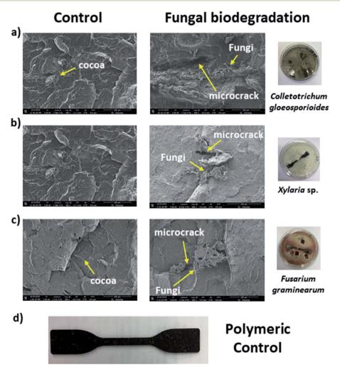
Fig. 2 Micrographs of SEM analysis of microbial biodegradation experiments using the bioplastic with 20% of cocoa after 75 days. The polymeric controls are shown in the left (a) *C. gloeosporioides* biodegradation; (b) *Xylaria* sp. biodegradation; (c) *F. graminearum* biodegradation; (d) polymeric control – HDPE/cocoa (80 : 20) composition.
