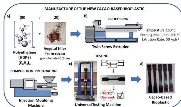
Fig. 1 Manufacturing process of new cacao-based bioplastic. (a) The bioplastic was manufactured using high density polyethylene (HDPE) and cacao shells as vegetal filler in the proportion 80 : 20, respectively; (b) the raw material was processed in a twin screw extruder and the composition was molded in an injection molding machine Romi Pratica 130 model; (c) tests of tensile behavior were performed in accordance to the ISO 527 standard; (d) samples of the new cacao-based-bioplastic.
