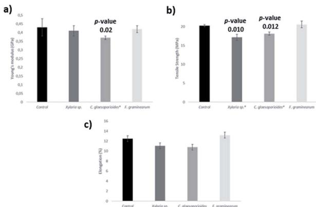
Fig. 4 Traction test parameters of the inoculated fungi after 75 days. (a) Young's modulus; (b) tensile strength; (c) elongation. \*Means indicate the significant statistical difference ( $p$ -value  $< 0.05$ ) in relation to the control, according to  $T$ -tests.
