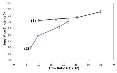
Fig. 11 Separation efficiency versus flow ratio for the microdevice with (1) the activated and (2) the non-activated triple-sided film valve at an inflow bacterial cell concentration of  $2 \times 10^7$  cells per ml.
