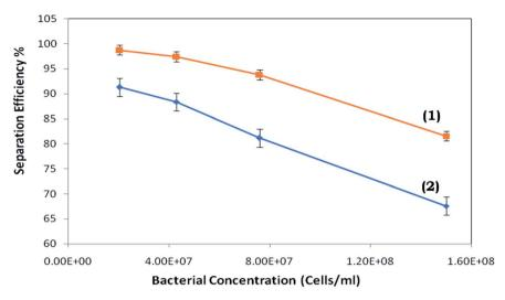
Fig. 8 Separation efficiency *versus* bacterial cell concentration for the microdevice with (1) the activated and (2) non-activated triple-sided film valve at a flow rate corresponding to the maximum efficiency.
