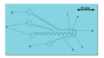
Fig. 1 Top view of the schematic diagram of the novel microfluidic device for filterless and continuous water purification: (a) input reservoir for the device, (b) impure water microchannel width changing from 300  $\mu m$  to 150  $\mu m$ , (c) pure water microchannel (200  $\mu m$ ), (d) U-shaped curve microchannel, (e) constriction (150  $\mu m$ ), (f) expansion (600  $\mu m$ ), (g) output reservoir for impure water, (h) output reservoir for pure water.
