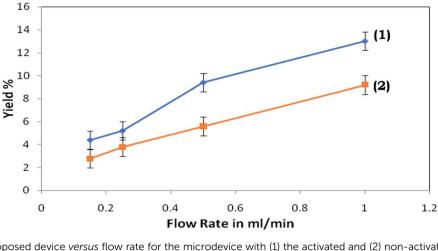
Yield% of the proposed device versus flow rate for the microdevice with (1) the activated and (2) non-activated triple-sided film valve.
