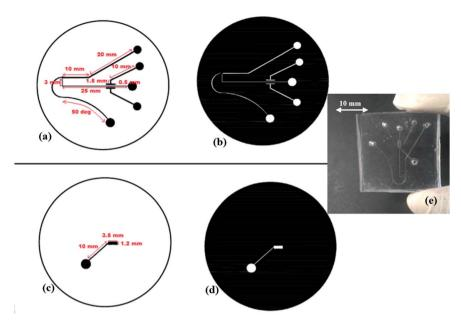
Fig. 3 (a) Schematic diagram of the mask used for the microfabrication process of generating the apparatus and method for the separation of suspended particles present in the liquid. The proposed masks in (a) and (b) were used for fabricating the 1st layer and the masks in (c) and (d) were used for fabricating the 2nd layer of the micro-valve structure, (e) micrograph of the fabricated device.
