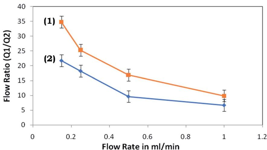
Fig. 9 Flow ratio versus flow rate for the microdevice with (1) the activated and (2) non-activated triple-sided film valve.
