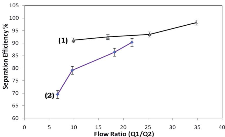
Fig. 11 Separation efficiency versus flow ratio for the microdevice with (1) the activated and (2) the non-activated triple-sided film valve at an inflow bacterial cell concentration of  $2 \times 10^7$  cells per ml.
