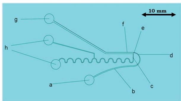
Fig. 1 Top view of the schematic diagram of the novel microfluidic device for filterless and continuous water purification: (a) input reservoir for the device, (b) impure water microchannel width changing from 300  $\mu\text{m}$  to 150  $\mu\text{m}$ , (c) pure water microchannel (200  $\mu\text{m}$ ), (d) U-shaped curve microchannel, (e) constriction (150  $\mu\text{m}$ ), (f) expansion (600  $\mu\text{m}$ ), (g) output reservoir for impure water, (h) output reservoir for pure water.
