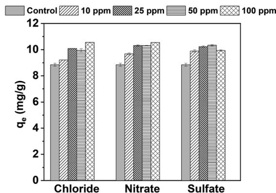
**Fig. 9** Effect of co-existing ions on the adsorption of phosphate. Initial phosphate concentration:  $5 \text{ mg L}^{-1}$ ; adsorbent dosage:  $0.5 \text{ g L}^{-1}$ ; pH: 7.0; contact time: 60 min. The control is phosphate uptake without co-existing ions.**Table 5** Phosphate removal from TSE
