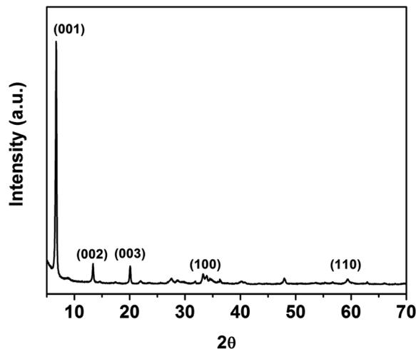
Fig. 2 Powder X-ray diffraction pattern of LZH.
