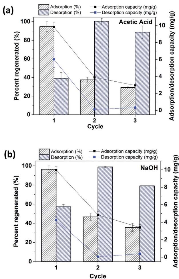
Fig. 10 Regeneration behavior LZH with (a) acetic acid and (b) NaOH regenerants. Initial phosphate concentration: 5  $\text{mg L}^{-1}$ ; adsorbent dosage: 0.5  $\text{g L}^{-1}$ ; pH: 7.0 (for adsorption); adsorption/desorption time: 60 min. The left scale is for the columns (adsorption/desorption in percent (%)) and the right scale is for the line + symbol (adsorption capacity in  $\text{mg g}^{-1}$ ).
