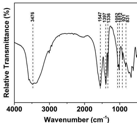
Fig. 5 FTIR spectra of the synthesized LZH.
