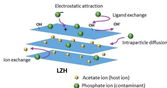
**Fig. 12** Proposed mechanisms of phosphate adsorption on LZH.
