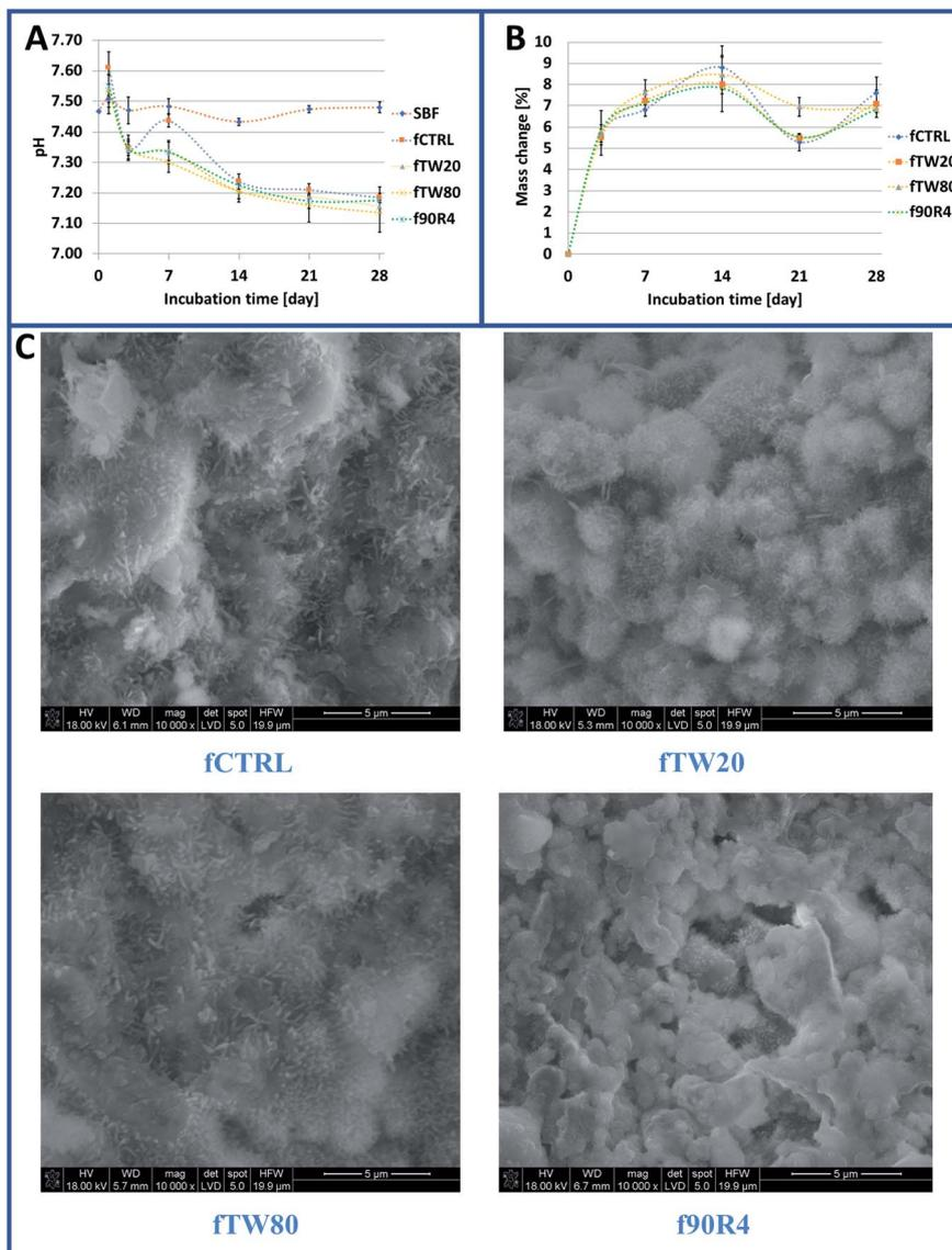
Fig. 10 (A) Changes of pH during cements incubation in SBF. (B) Materials' mass changes after incubation in SBF in selected time points. (C) Microstructure of cross-sections of the investigated cements after 7 day incubation in SBF (magnification 10 000 $\times$ ).
