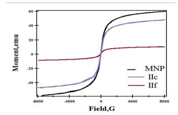
Fig. 6 Magnetization curves of MNP, II<sub>c</sub>, and II<sub>f</sub>
