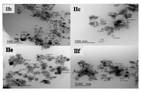
Fig. 8 TEM images of the hydrogel nanocomposites.
