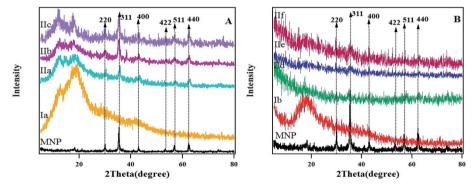
Fig. 4 XRD patterns of MNPs, hydrogel  $I_{a,b}$  and their nanocomposites  $II_{a-f}$ .
