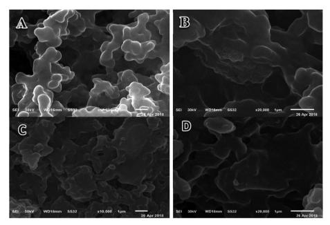
Fig. 7 SEM images of hydrogel I<sub>a</sub> (A, B) and magnetic hydrogel nanocomposite II<sub>c</sub> (C, D).
