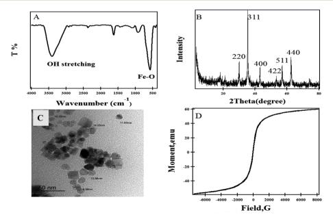
Fig. 2 (A) FTIR spectrum, (B) XRD pattern, (C) TEM of MNP and (D) magnetization versus the applied magnetic field at room temperature of MNPs.
