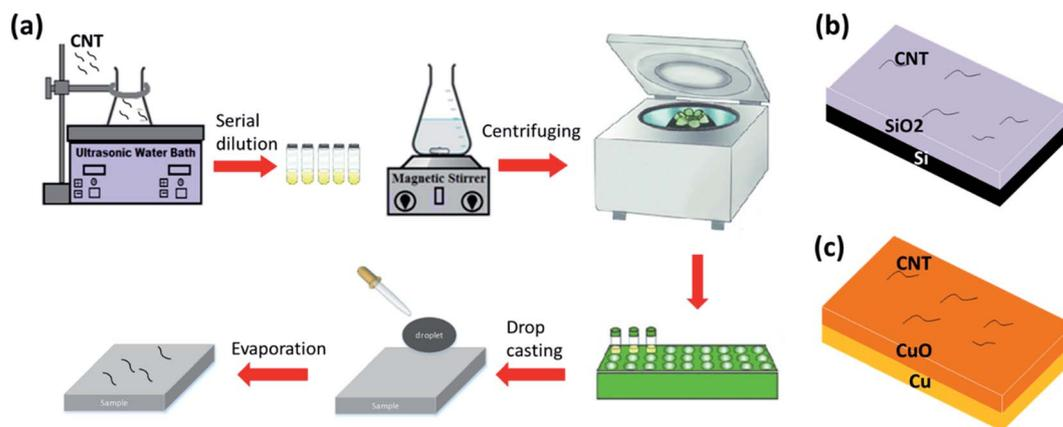
Fig. 1 (a) Steps for the dispersion of CNT powder and sample preparation, (b) schematic of the first device using Si as a substrate with a thin SiO<sub>2</sub> layer of 2.31 nm, (c) schematic of the second device using Cu sheet as the substrate with a thin CuO layer of 3.69 nm.
