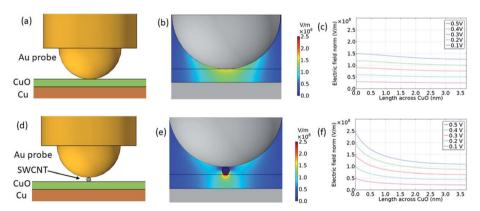
Fig. 7 (a) COMSOL simulation model for Au probe on CuO/Cu sample. (b) The electric field distribution at the interface. (c) The electric field profile along a vertical middle line a cross CuO layer, at different applied voltages. (d) COMSOL simulation model for Au probe on CNT/CuO/Cu sample. (e) The electric field distribution at the interface. (f) The electric field profile along a vertical middle line a cross CuO layer, at different applied voltages
