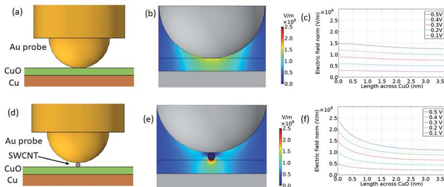
**Fig. 7** (a) COMSOL simulation model for Au probe on CuO/Cu sample. (b) The electric field distribution at the interface. (c) The electric field profile along a vertical middle line a cross CuO layer, at different applied voltages. (d) COMSOL simulation model for Au probe on CNT/CuO/Cu sample. (e) The electric field distribution at the interface. (f) The electric field profile along a vertical middle line a cross CuO layer, at different applied voltages.
