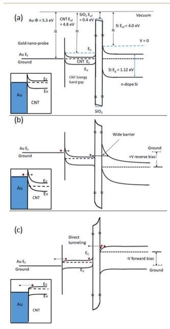
Fig. 8 Schematics of the energy band diagram of  $Au/CNT/SiO_2/Si$ . (a) At zero bias. (b) Reverse (positive) bias. (c) Forward (negative) bias. With inset showing a simplified nano Schottky junction between Au and CNT.
