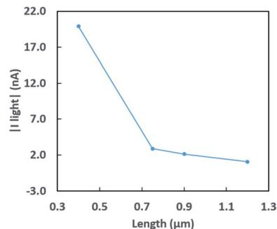
Fig. 5 Variation of the light current at a reading voltage of (−1 V) for Au/CNT/SiO<sub>2</sub>/Si device as a function of CNT length extracted from AFM topography images.
