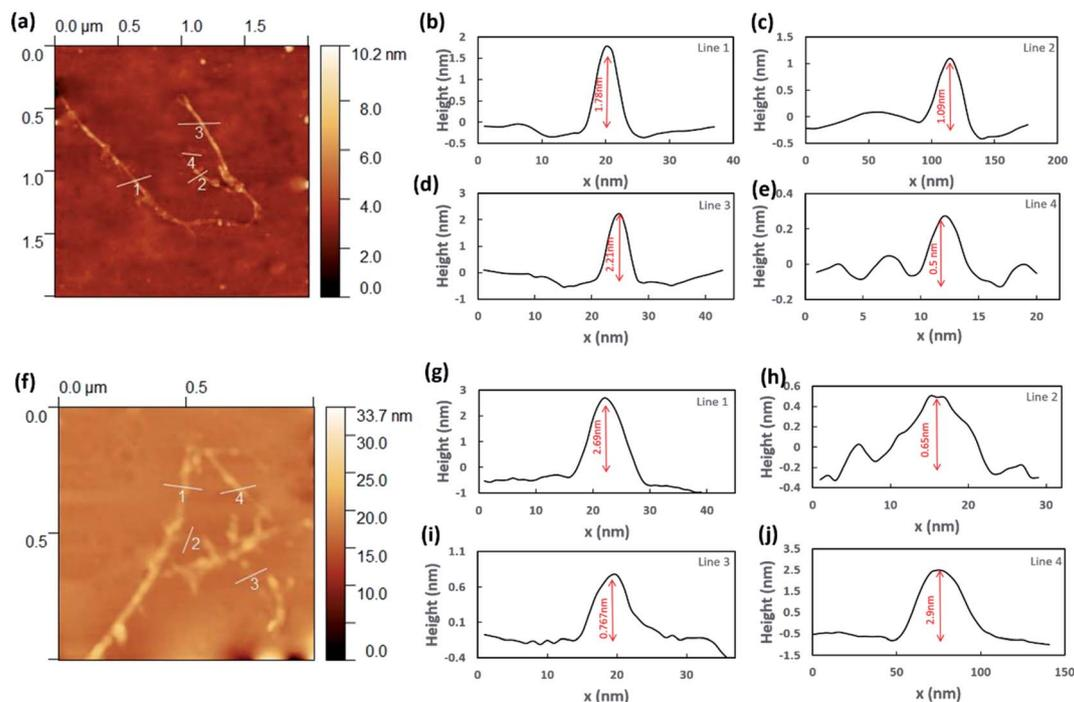
Fig. 3 (a) AFM topography image and the corresponding diameter distribution along: (b) line 1, (c) line 2, (d) line 3, (e) line 4, (f) AFM topography image and the corresponding diameter distribution along: (g) line 1, (h) line 2, (i) line 3, (j) line 4. The average diameter of SWCNT is 2.2 nm.
