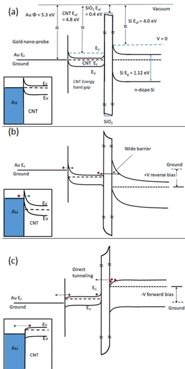
Fig. 8 Schematics of the energy band diagram of Au/CNT/SiO<sub>2</sub>/Si. (a) At zero bias. (b) Reverse (positive) bias. (c) Forward (negative) bias. With inset showing a simplified nano Schottky junction between Au and CNT.
