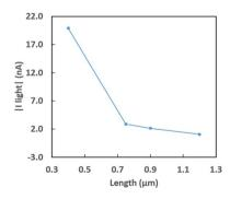
Fig. 5 Variation of the light current at a reading voltage of (-1 V) for Au/CNT/SiO<sub>2</sub>/Si device as a function of CNT length extracted from AFM topography images.
