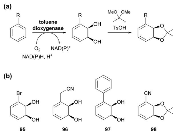
Scheme 15 Arene *cis*-dihydroxylation by toluene dioxygenase (TDO): (a) general reaction scheme for the dihydroxylation of a mono-substituted arene by TDO and for the conversion of the resulting diol into an acetonide. (b) Examples of commercially available arene *cis*-dihydrodiols or the corresponding acetonides (as of January 2021).
