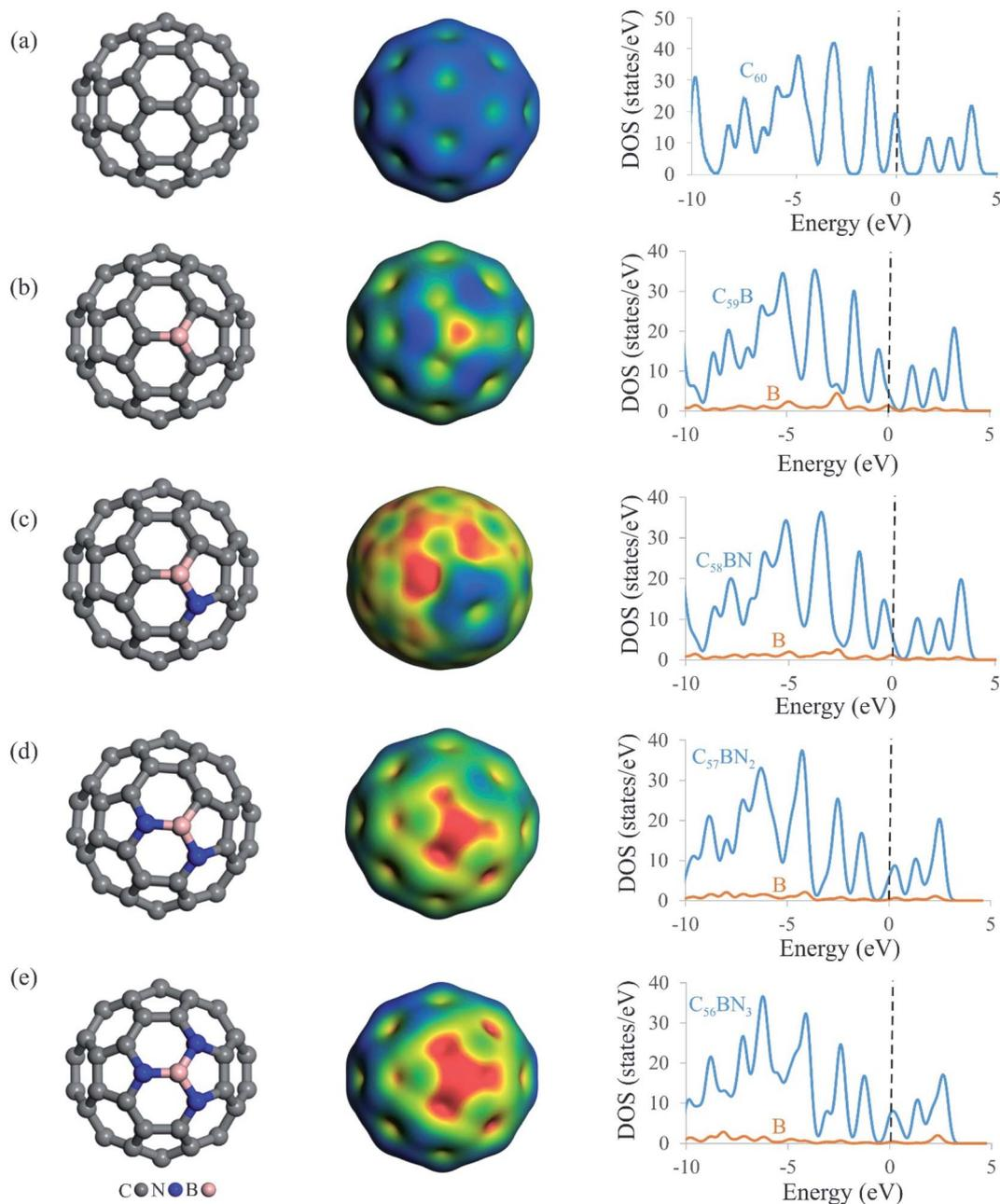
**Fig. 1** Local atomic structures (left) molecular electrostatic potential isosurfaces (MEP, middle) and TDOS plots (right) of (a)  $C_{60}$ , (b)  $C_{59}B$ , (c)  $C_{58}BN$ , (d)  $C_{57}BN_2$  and (e)  $C_{56}BN_3$ . The dashed line in TDOS plots shows the Fermi level. The color range in the MEP maps is from blue (more negative =  $-0.001$  a.u.) to red (more positive =  $0.078$  a.u.).
