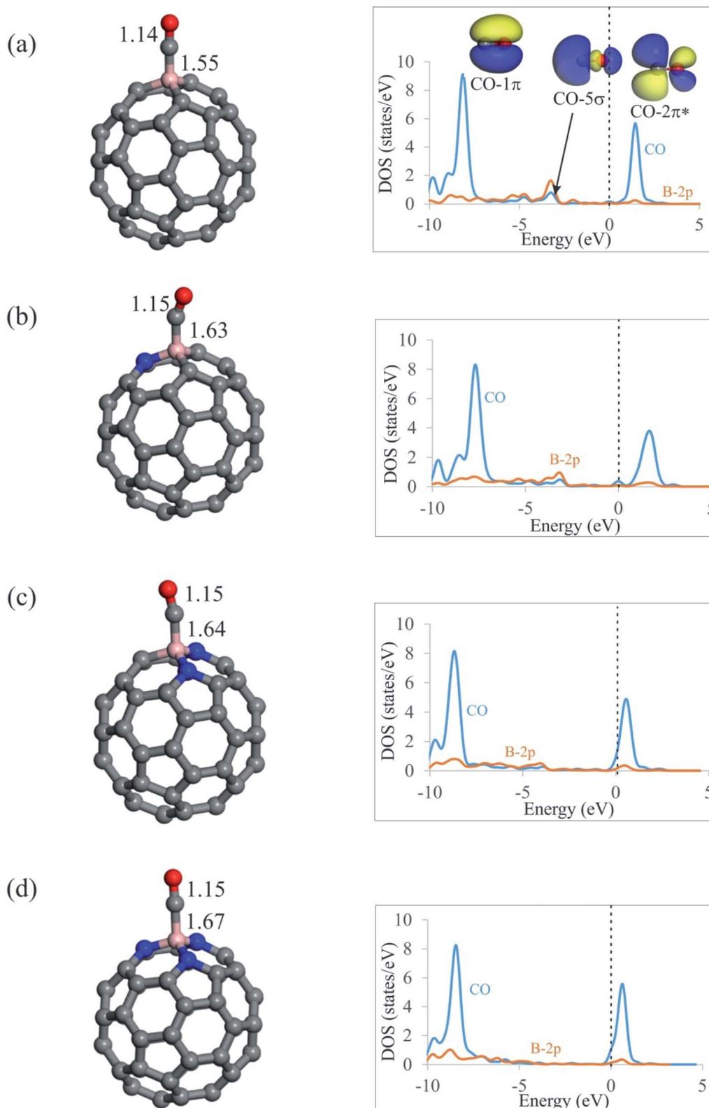
Fig. 3 The optimized local atomic structures, binding distances (in Å), and PDOS plots of CO adsorbed onto (a) C<sub>59</sub>B, (b) C<sub>58</sub>BN, (c) C<sub>57</sub>BN<sub>2</sub> and (d) C<sub>56</sub>BN<sub>3</sub> fullerenes. In the PDOS plots, the Fermi level is indicated by the dashed line.
