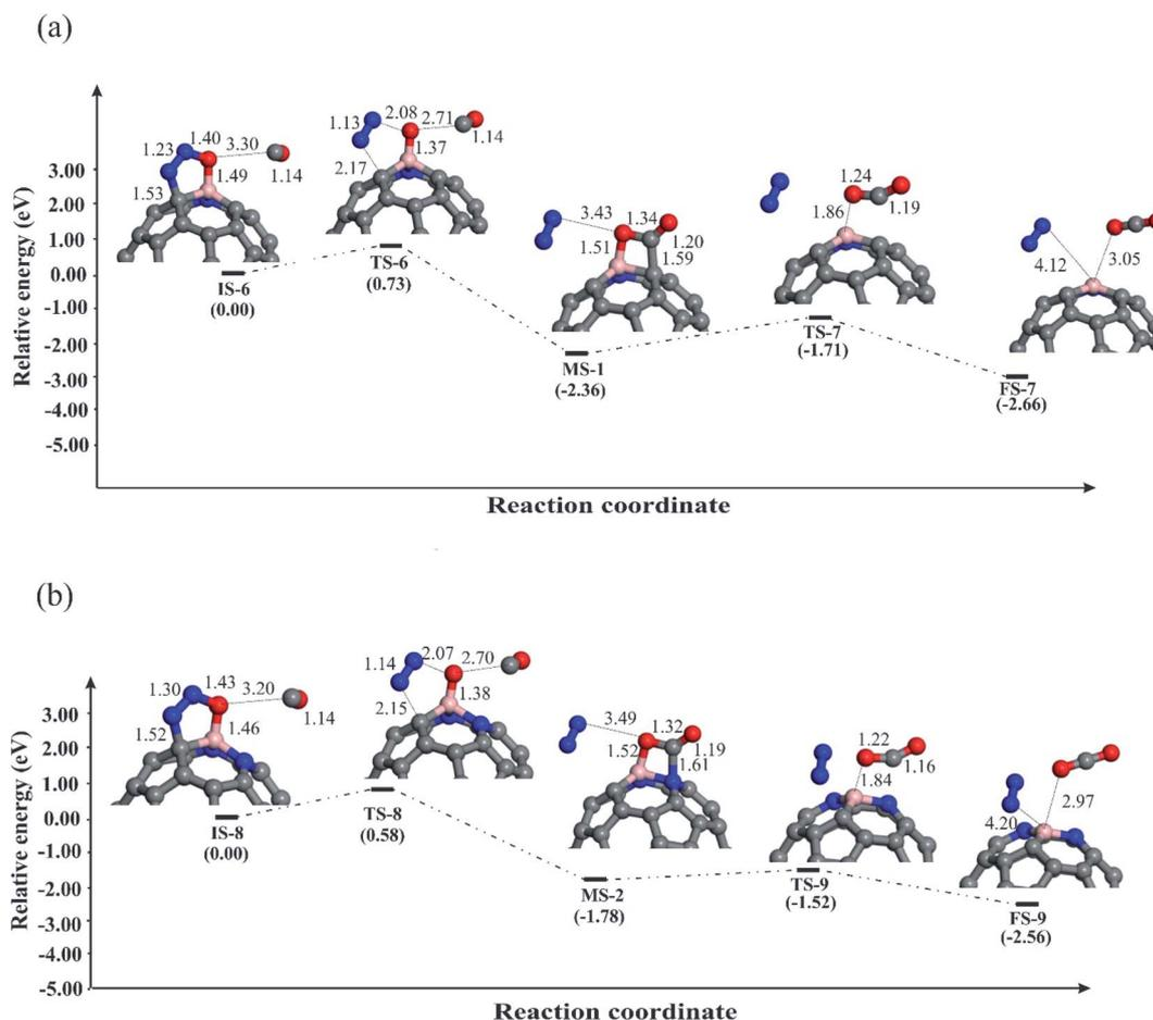
Fig. 6 The potential energy diagram and relevant bond distances (in Å) for reduction of  $\text{N}_2\text{O}$  by CO molecule through the L–H mechanism over (a)  $\text{C}_{58}\text{BN}$  and (b)  $\text{C}_{57}\text{BN}_2$  fullerenes.
