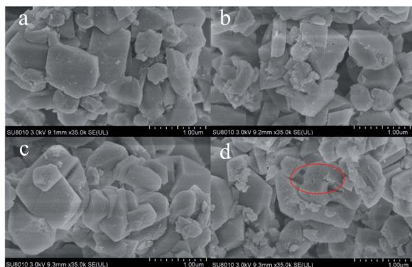
Fig. 3 SEM images of USY samples before (pristine USY) and after the alkali treatment at different concentrations. ((a) Pristine USY; (b) 0.1 mol L<sup>-1</sup> NH<sub>4</sub>OH; (c) 0.2 mol L<sup>-1</sup> NH<sub>4</sub>OH; (d) 0.1 mol L<sup>-1</sup> NaOH).
