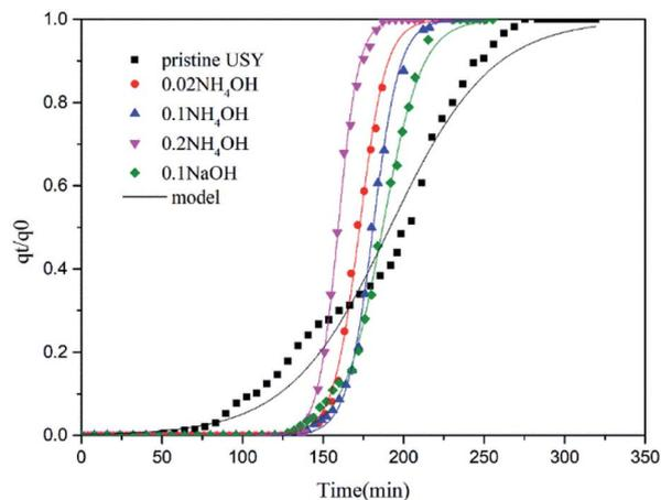
Fig. 5 Breakthrough curves and mathematic model for USY samples before (pristine USY) and after the alkali treatment.
