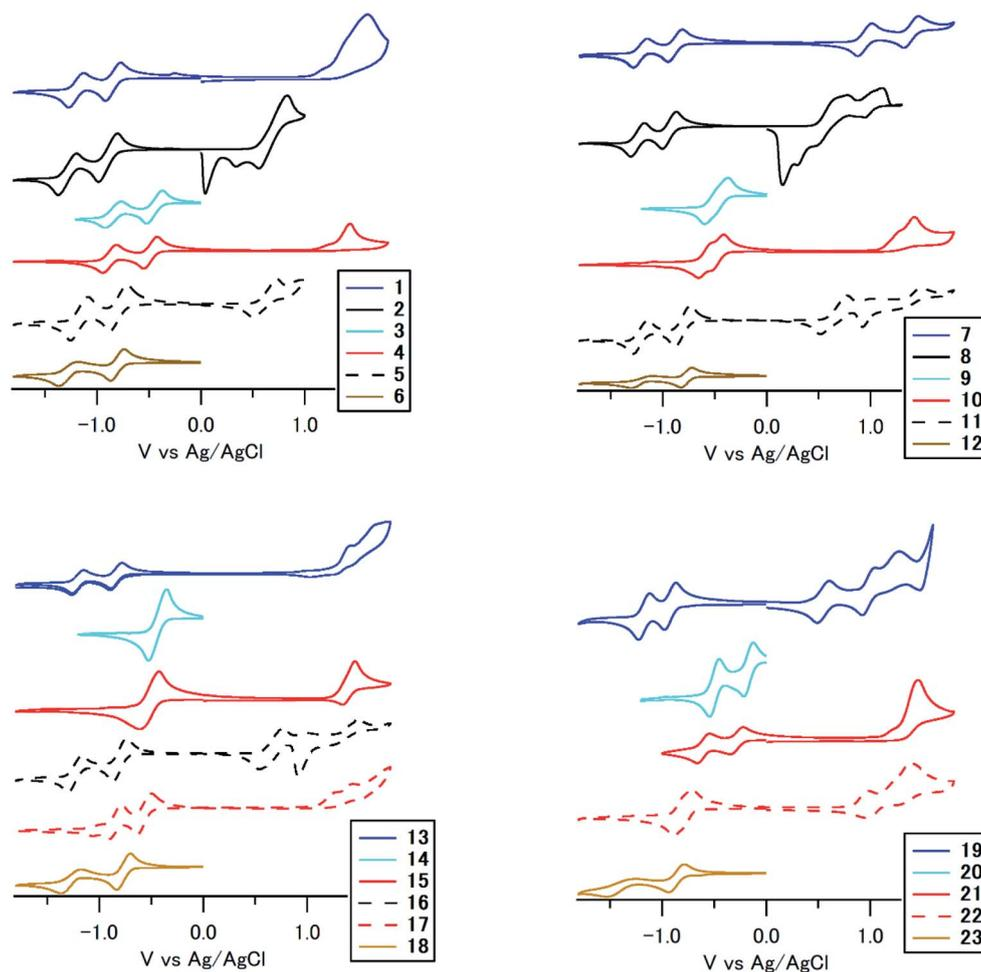
Fig. 6 Cyclic voltammograms of 1–23 measured in  $\text{CH}_2\text{Cl}_2$  classified according to the substitution position. The color was determined by the introduced substituent. The dotted line indicates monochloro-monosubstituted derivatives or diamino-disubstituted derivative.
