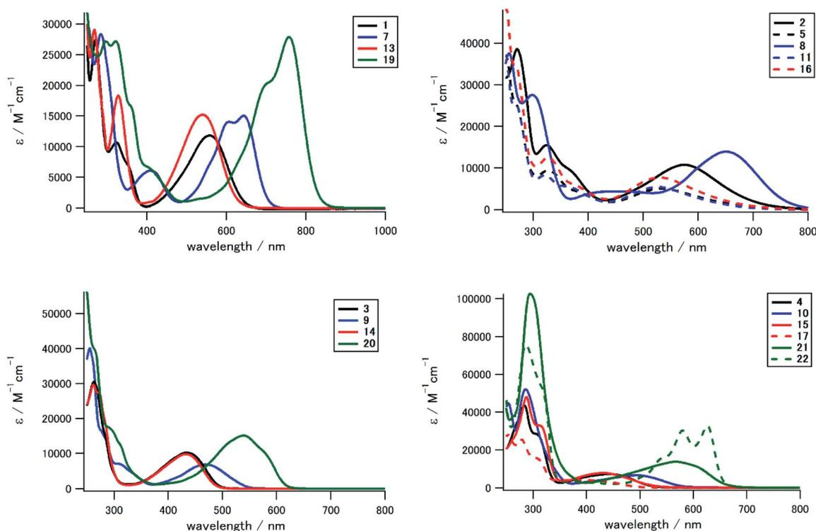
Fig. 4 UV-Vis spectra of 1–22 in  $\text{CH}_2\text{Cl}_2$  classified according to the substituent. The color was determined by the position of the introduced substituent. The dotted line indicates monochloro-monosubstituted derivatives or diamino-disubstituted derivative.
