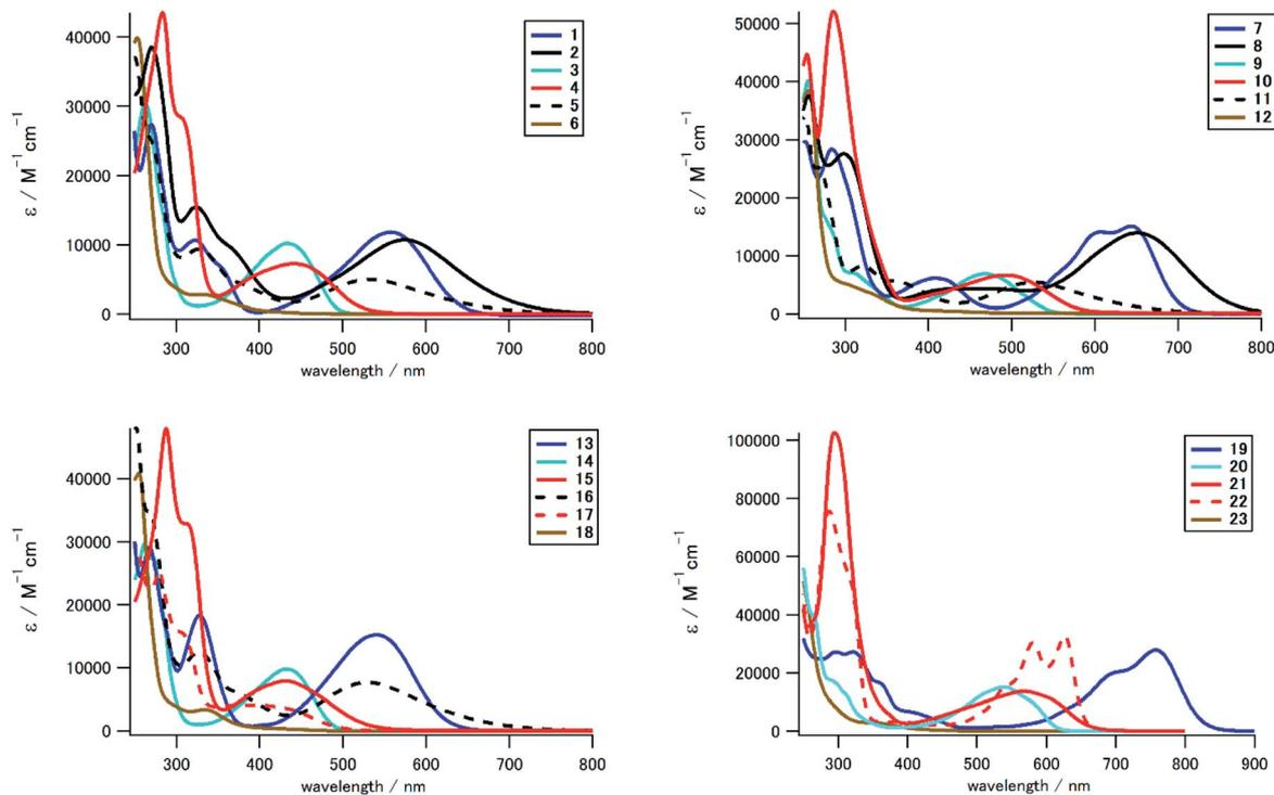
Fig. 3 UV-Vis spectra of 1–23 in  $\text{CH}_2\text{Cl}_2$  classified according to the substitution position. The color was determined by the introduced substituent. The dotted line indicates monochloro-monosubstituted derivatives or diamino-disubstituted derivative.
