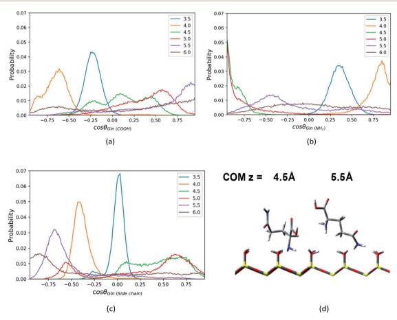
Fig. 7 The probability distributions of  $\cos \theta$ , where  $\theta$  is the angle between the normal direction z of silica surface and (a)  $C_1 - C_2$  vector or (b)  $C_1 - N_1$  vector or (c)  $C_1 - N_2$  vector in the Gln molecule, at the distance = 3.5 - 6.0 Å from the surface in direction of z axis. (d) The representative configurations of the Gln molecule at z = 4.5 Å and 5.5 Å.
