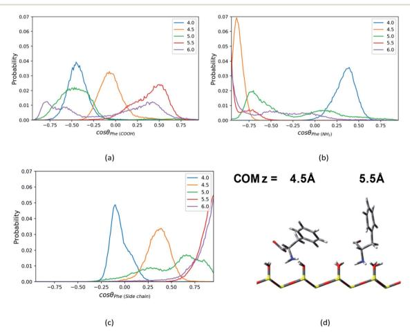
Fig. 5 The probability distributions of  $\cos \theta$ , where  $\theta$  is the angle between the normal direction z of silica surface and (a)  $C_1 - C_2$  vector or (b)  $C_1 - C_3$  vector or (c)  $C_1 - C_3$  vector in the Phe molecule, at the distance = 4.0 - 6.0 Å from the surface in direction of z axis. (d) The representative configurations of the Phe molecule at z = 4.5 Å and 5.5 Å.
