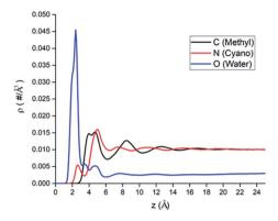
Fig. 2 The atomic number density profiles of water-ACN binary mixture solvent with different atomic representations: black, red and blue line represent the methyl carbon atom, the nitrogen atom of ACN and the oxygen atom of water, respectively.
