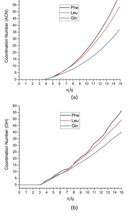
Fig. 4 (a) The coordination number for ACN at the most stabilized state around each amino acid as a function of the distance between the β-carbon atom of each amino acid and methyl carbon atoms from ACN molecules. (b) The coordination number for hydroxyl groups in solvent system (water molecules and silanol groups) at the most stabilized state around each amino acid as a function of the distance between the α-carbon atom of each amino acids and oxygen atoms of hydroxyl groups.
