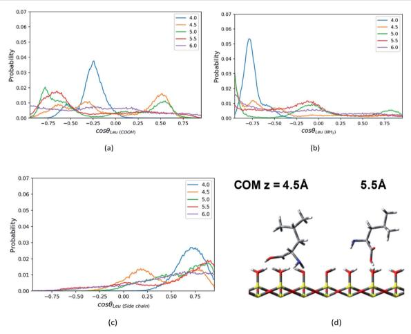
Fig. 6 The probability distributions of  $\cos \theta$ , where  $\theta$  is the angle between the normal direction z of silica surface and (a)  $C_1 - C_2$  vector or (b)  $C_1 - C_1$  vector or (c)  $C_1 - C_4$  vector in the Leu molecule, at the distance = 4.0–6.0 Å from the surface in direction of z axis. (d) The configurations of a Leu molecule at z = 4.5 Å and 5.5 Å.
