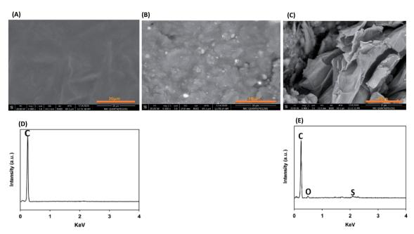
Fig. 1 (A–C) SEM images of (A) RGR' smooth region, (B) RGR' rough region, and (C) FEGR electrodes. (D and E) EDX analysis of RGR' smooth region (D) and FEGR (E) electrodes, respectively.
