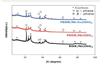
Fig. 7 XRD patterns for RGR/Ni(OH)<sub>2</sub> (black line), FEGR/Ni(OH)<sub>2</sub> (red line), and FEGR/Ni-Co(OH)<sub>2</sub> (blue line) films
