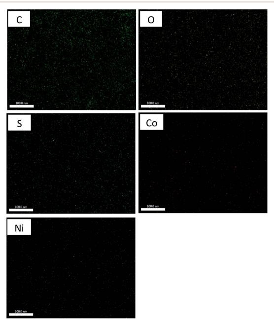
Fig. 6 Elemental mapping EDX analysis of FEGR/Ni-Co(OH)<sub>2</sub> film.
