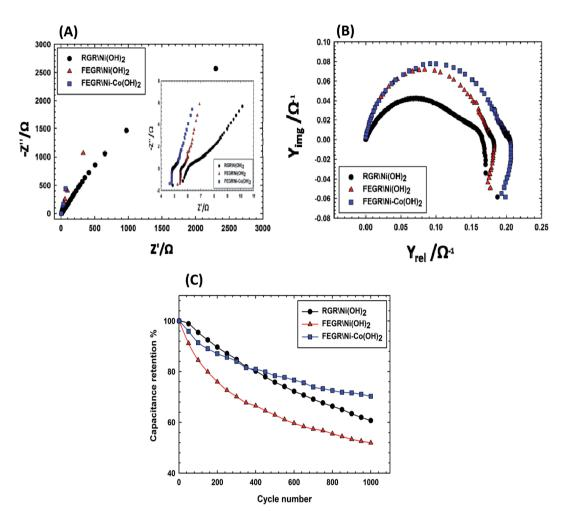
Fig. 9 (A) Nyquist plots of RGR/Ni(OH)<sub>2</sub>, FEGR/Ni(OH)<sub>2</sub>, and FEGR/Ni–Co(OH)<sub>2</sub> films at OCP and their insets at high frequencies. (B) Admittance plots of RGR/Ni(OH)<sub>2</sub>, FEGR/Ni(OH)<sub>2</sub>, and FEGR/Ni–Co(OH)<sub>2</sub> films. (C) Stability curves of RGR/Ni(OH)<sub>2</sub>, FEGR/Ni(OH)<sub>2</sub>, and FEGR/Ni–Co(OH)<sub>2</sub> films at a current density of 50 A  $g^{-1}$ .
