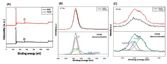
Fig. 2 XPS analysis of RGR (black line), and FEGR (red line) electrodes: (A) survey, (B) enlarged view of C 1s, and (C) enlarged view of O 1s.
