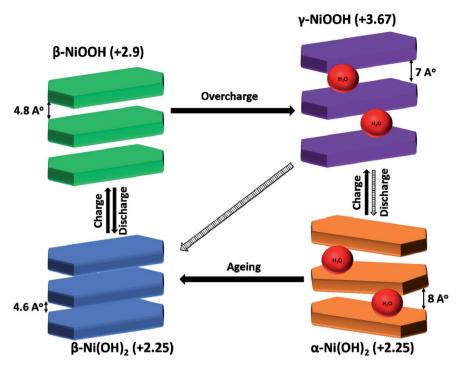
Scheme 1 Schematic illustration of Ni(OH)<sub>2</sub>/NiOOH phase transformation (Bode diagram).<sup>42</sup>
