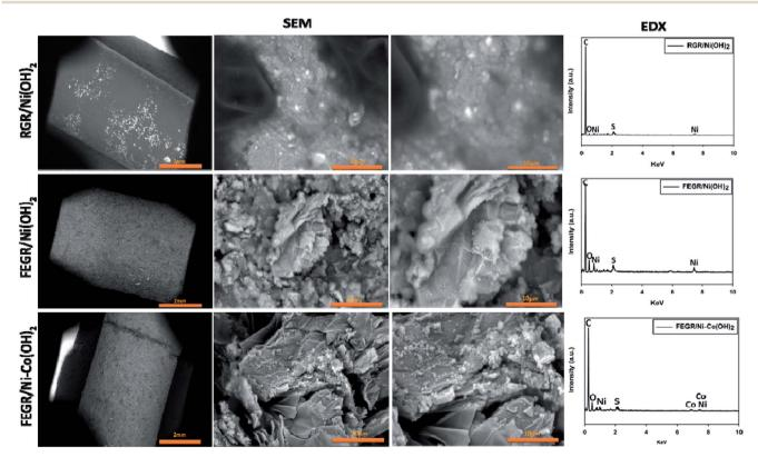
SEM images with different magnifications and EDX analysis of RGR/Ni(OH)<sub>2</sub>, FEGR/Ni(OH)<sub>2</sub>, and FEGR/Ni–Co(OH)<sub>2</sub> film electrodes.
