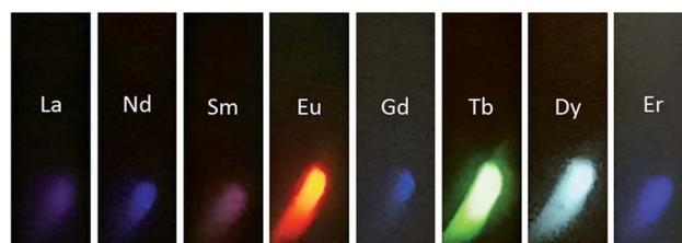
Fig. 3 Pictures of ZnAlRE<sub>5%</sub>-BTC-P123 samples exposed to UV radiation (290 nm).
