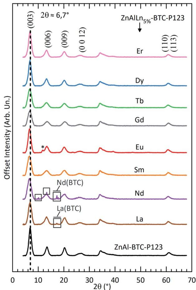
Fig. 1 Powder X-ray diffraction patterns of  $\text{ZnAl-BTC-P123}$  and  $\text{ZnAlLn}_{5\%}\text{-BTC-P123}$  ( $\text{Ln} = \text{La}$  and from  $\text{Nd}$  to  $\text{Er}$ ). The Bragg peaks inside the rectangles are attributed to the formation of the respective  $\text{Ln}(\text{BTC})$  complex.<sup>35–37</sup> The starred peak are ascribed to a carbonate-intercalated LDH phase formed in the  $\text{Eu}^{3+}$ -containing solid.
