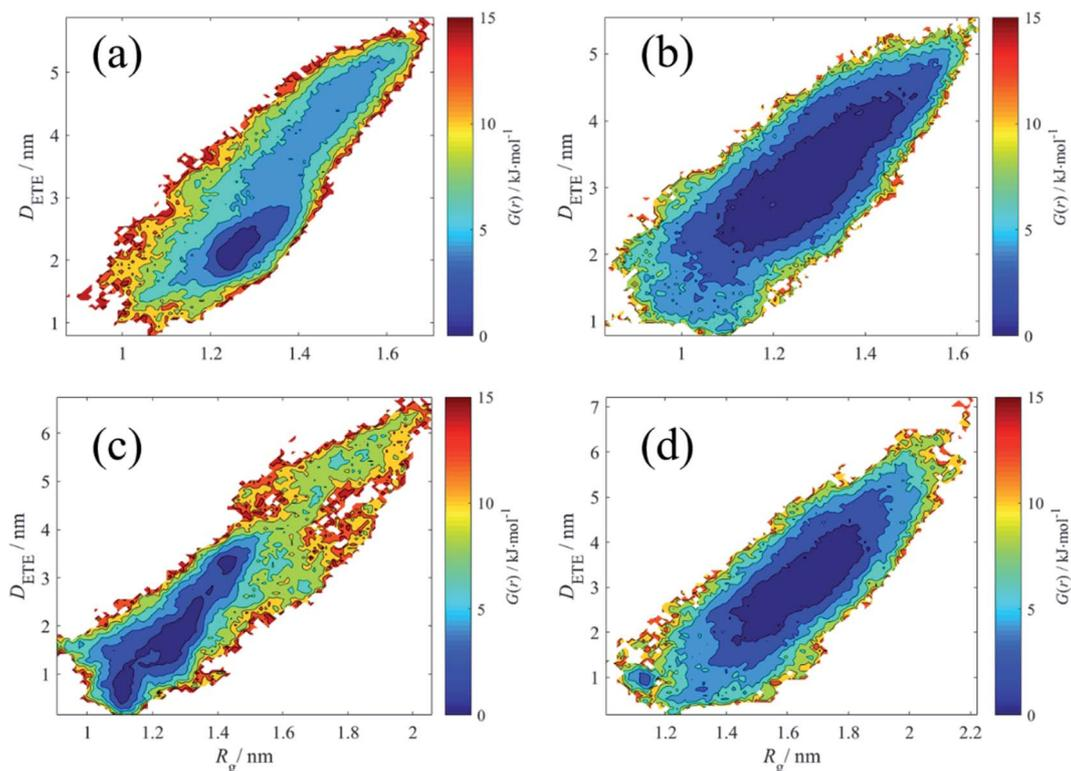
Fig. 9 The free energy (in  $\text{kJ mol}^{-1}$ ) contour explored in the radius of gyration and end-to-end distance. (a) HPAM30\_dot; (b) HPAM30\_solo; (c) HPAM40\_dot; (d) HPAM40\_solo.
