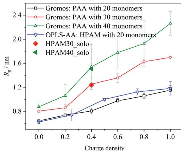
Fig. 2 The comparison of average radius of gyration of HPAM and PAA chains simulated by OPLS-AA and Gromos53a6 force field, respectively.
