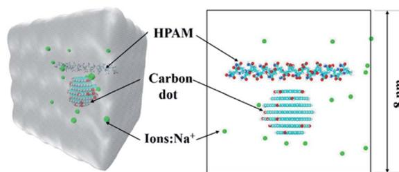
Fig. 1 The initial configuration of the HPAM40\_dot system (blue: nitrogen atoms; red and white: oxygen and hydrogen atoms, respectively; cyan: carbon; green: Na<sup>+</sup> ions, water is not plotted in).
