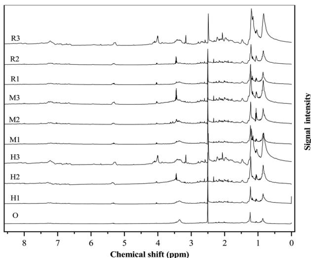
Fig. 4 <sup>1</sup>H NMR spectra of bio-oils.
