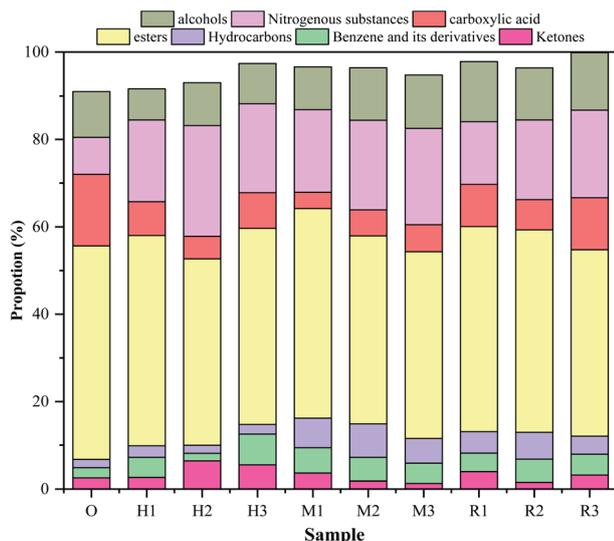
Fig. 3 Effect of catalyst on the chemical composition of bio-oil.
