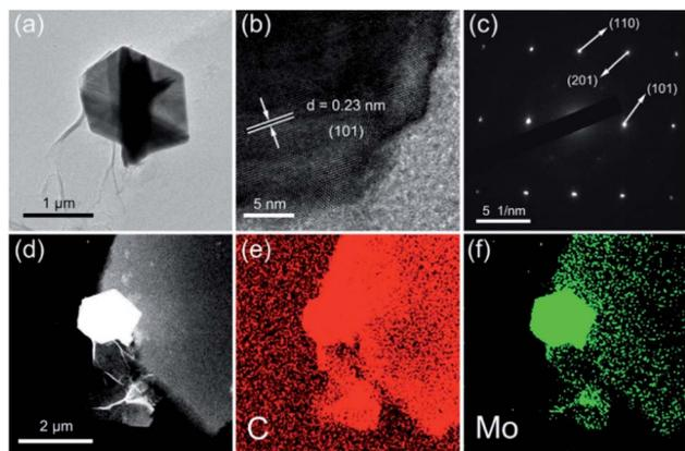
Fig. 4 (a) TEM and (b) HR-TEM images of Mo<sub>2</sub>C/C-2; (c) SAED pattern of the Mo<sub>2</sub>C/C-2; EDS mapping images of (d) the Mo<sub>2</sub>C/C-2 and the elements of (e) C, (f) Mo, respectively.
