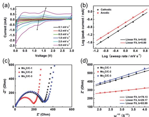
Fig. 6 (a) CV curves of Mo<sub>2</sub>C/C-2 at sweep rates from 0.1 to 5.0 mV s<sup>-1</sup>; (b) relationship between the peak currents and scan rates in their logarithmic format for Mo<sub>2</sub>C/C-2; (c) Nyquist plots of Mo<sub>2</sub>C/C-1, Mo<sub>2</sub>C/C-2 and Mo<sub>2</sub>C/C-3 at fresh coin cells; (d) corresponding linear fits of the *Z'* versus  $\omega^{-1/2}$  in the low-frequency region.
