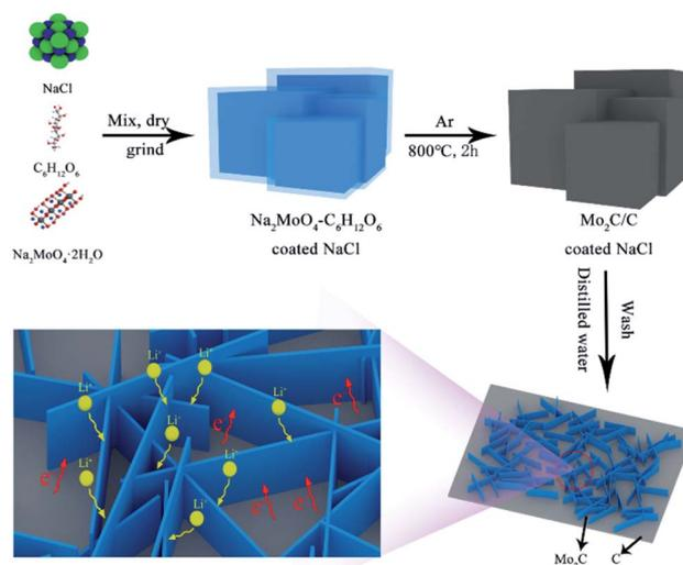
Fig. 1 Schematic illustration of fabrication of hierarchical Mo<sub>2</sub>C/C nanosheet composite.
