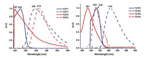
Fig. 3 Normalized UV-vis absorption ( $C_M = 10^{-7}$  M in THF, solid lines) and emission ( $C_M = 10^{-8}$  M in THF, dotted lines) spectra of: (A) TCP1,4 (left) TCP2,5 (right) (absorption maxima were used as the excitation wavelengths).
