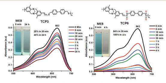
Fig. 6 Methylene blue (MEB) dye adsorption by TCP3,6 at various time intervals (insets: photographs showing the color change upon dye adsorption).
