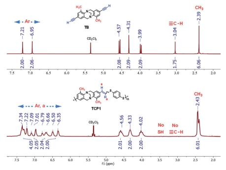
Fig. 1 Comparative <sup>1</sup>H-NMR of TB (up) and TCP1 (down).
