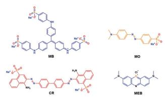
Fig. 4 Structures of methyl blue (MB), methyl orange (MO), congo red (CR), and methylene blue (MEB).
