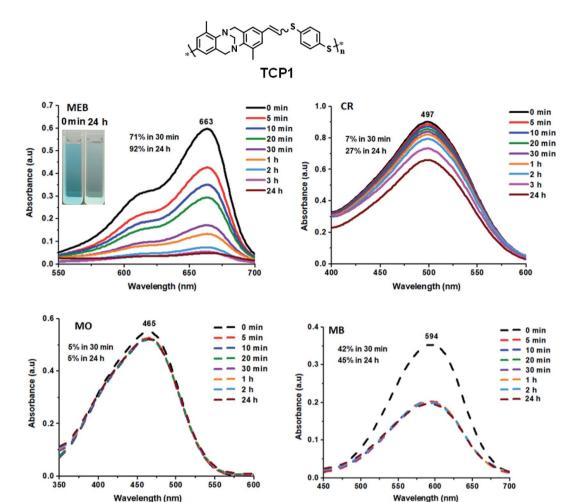
Fig. 5 TCP1 adsorption of methylene blue (MEB), Congo red (CR), methyl orange (MO), and methyl blue (MB) at various time intervals (inset: photographs showing the color change upon dye adsorption).
