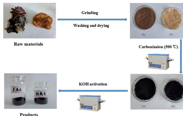
Fig. 1 Preparation process schematic of FAC<sub>X</sub> and HAC<sub>X</sub>.
