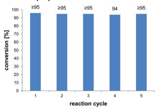
Fig. 3 Conversions of semi-preparative scale reactions of AmbDH3-CLEA with 1. The conversion was determined by  $^1\text{H}$  NMR spectroscopy. Reaction conditions: 33  $\mu\text{mol}$  (4 mM) of 1, 0.19 u AmbDH3-CLEA, 30 °C, 16 h.
